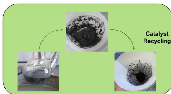
Figure I.1.0 Illustration of the Pd@TRGO-g-PETox catalyst recycling by thermal switching between dispersion and sedimentation behavior. [17]
