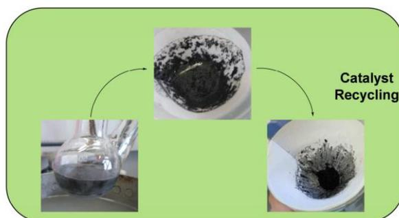
**Figure I.1.0** Illustration of the Pd@TRGO-g-PETox catalyst recycling by thermal switching between dispersion and sedimentation behavior.<sup>[17]</sup>
