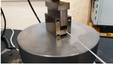
Figure 2.5: Single yarn compression device
