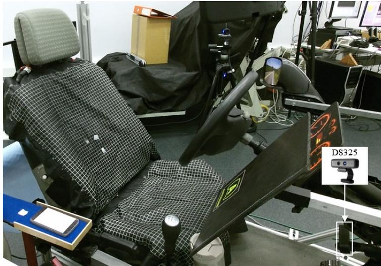
**Figure 6.3.** Depth camera DS325 is mounted above the pedals and right below the steering wheel to scan the legroom.
