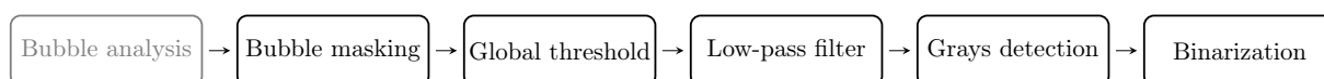
Figure 4.5: Block diagram of the image processing method for extracting the coordinates of the biological cell contour.
