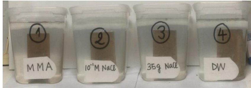
Fig. 7-1 Lime-treated specimens placed in four different fluids for 1 st wetting during the W-D cycles.
