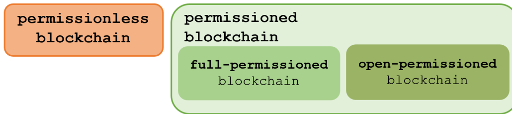
FIGURE 1.2 – The different participation modes characterizing blockchains and DLTs. After a first distinction based on the reading rights (i.e., permissionless and permissioned), the second distinction is based on writing rights of the data on the ledger.
