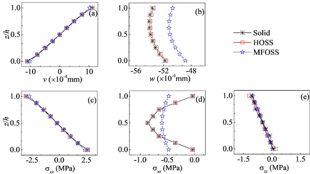
**Fig. 2.11.** Clamped square plate under distributed loading – Through-the-thickness displacements and stresses at point C, in the thick case.
