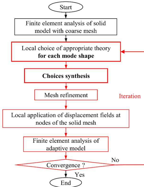
Fig. 4.6. Flowchart of adaptive modeling process for vibration analysis.
