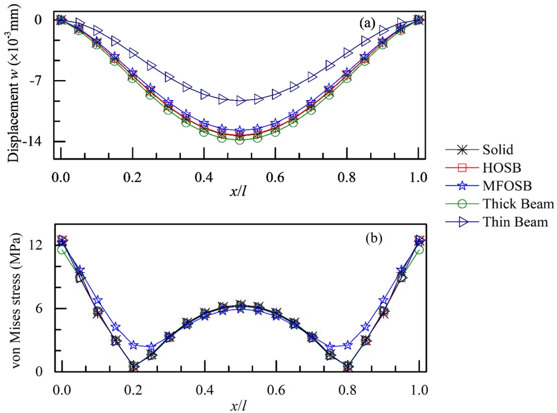
**Fig. 3.13.** Straight beam with square cross-section under distributed loading – Distribution of vertical displacement along the mid-axis (a) and von Mises stress along a line on the lower surface (b), in the thick case.
