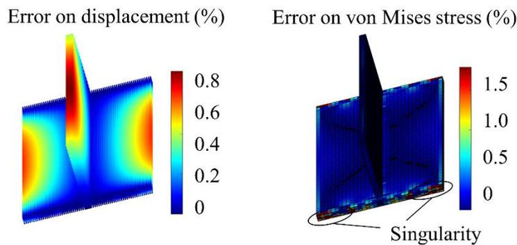
**Fig. 4.20.** “T” shape plates – Errors on displacement at each node and von Mises stress at the center of each element over the whole structure by comparing the optimal model and the reference solid model.
