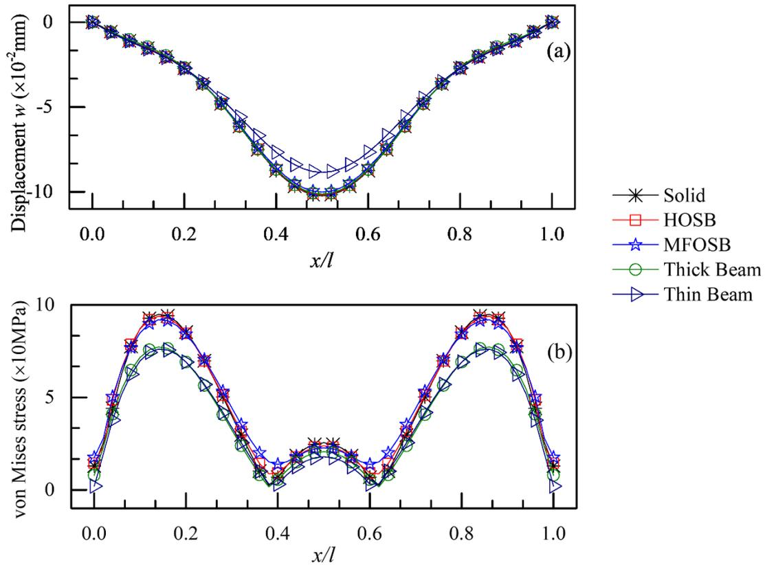
**Fig. 19.** Curved beam with square cross-section under distributed loading – Distribution of vertical displacement along the mid-axis (a) and von Mises stress along a line on the lower surface (b), in the thick case.
