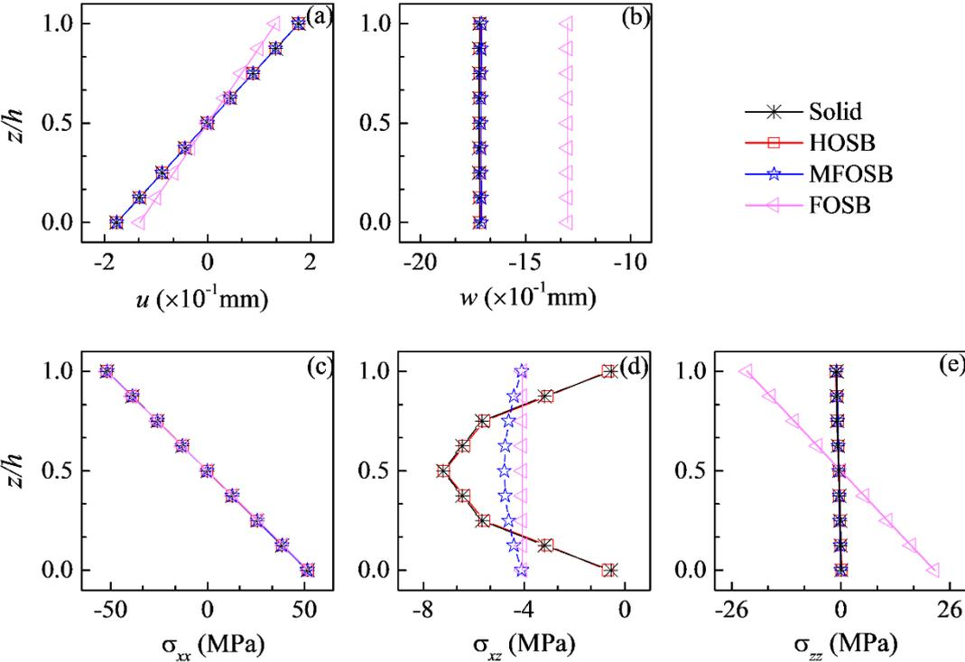
**Fig. 3.11.** Straight beam with square cross-section under distributed loading – Through-the-thickness displacement and stresses along a line  $JK$ , in the thin case.
