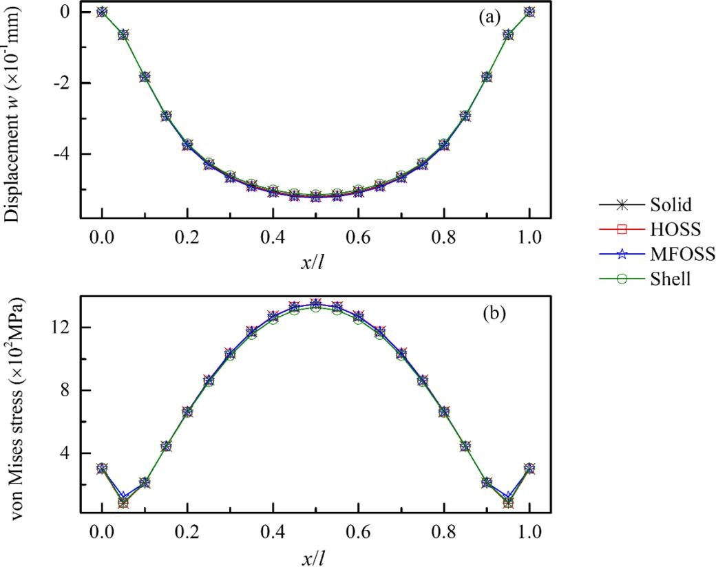
**Fig. 2.14.** Quarter of cylinder under pressure – Distribution of vertical displacement (a) and von Mises stress (b) along a line on the lower face, in the thin case.
