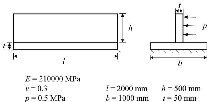
**Fig. 4.16.** “T” shape plates – Presentation of the example.
