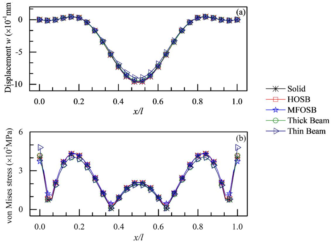
**Fig. 3.17.** Curved beam with square cross-section under distributed loading – Distribution of vertical displacement along the mid-axis (a) and von Mises stress along a line on the lower surface (b), in the thin case.
