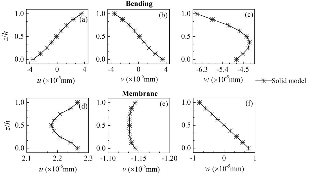
**Fig. 2.2.** Thick square plate under membrane or bending loading – Distribution of through-the-thickness displacements.
