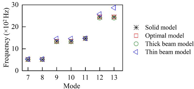
**Fig. 4.25.** Moderately thick structures – First seven natural frequencies for the beam models, optimal model and reference solid model in case 1.
