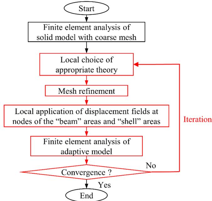
**Fig. 4.1.** Flowchart of the adaptive modeling process.
