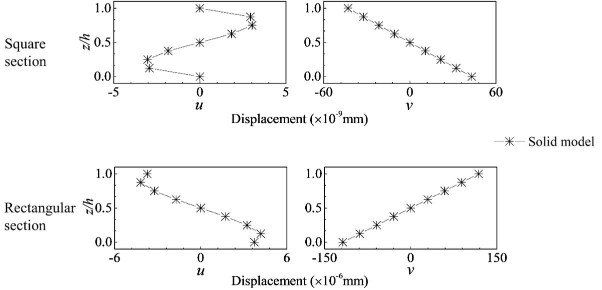
**Fig. 3.5.** Displacements of nodes through the thickness of spatial beam model for torsion.
