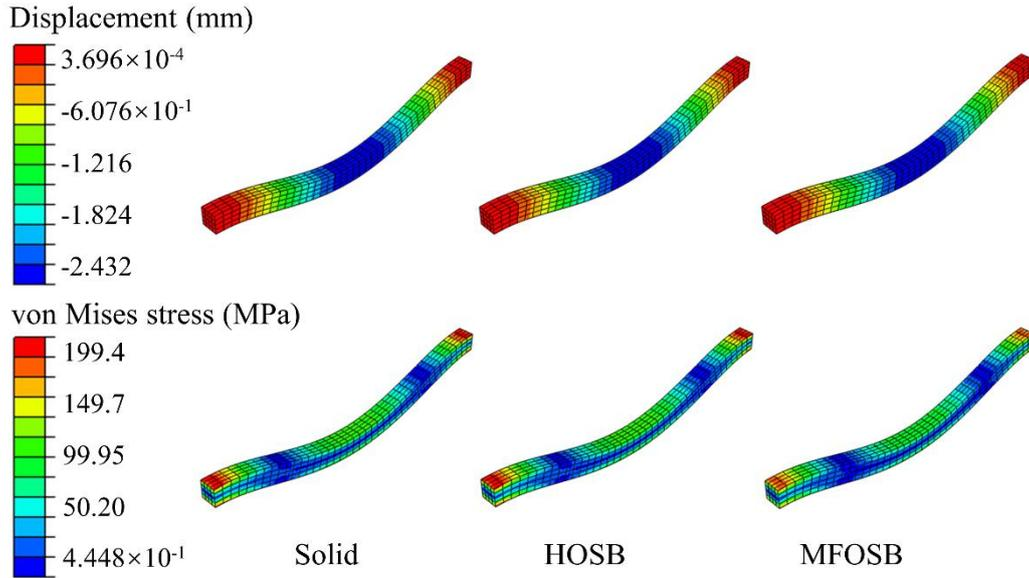
**Fig. 3.9.** Straight beam with square cross-section under distributed loading – Displacement  $w$  and von Mises stress distribution in the thin case.
