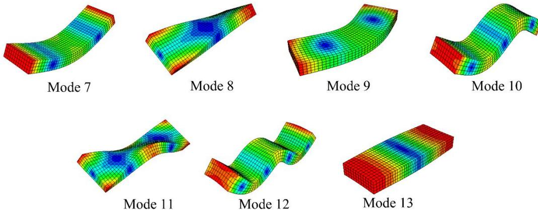
**Fig. 4.26.** Moderately thick structures – First seven mode shapes for a reference solid model in case 2.
