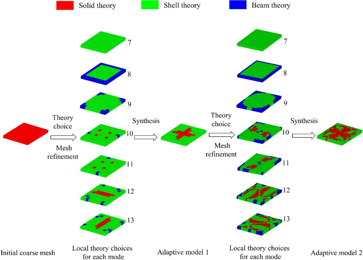
**Fig. 4.30.** Moderately thick structures – Theory choice for the first seven modes in case 3.
