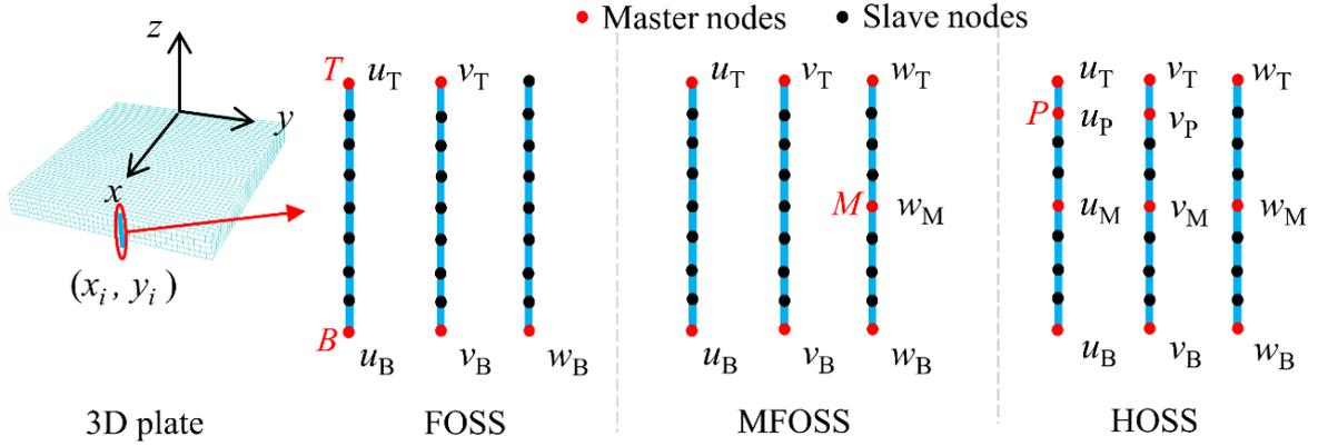
**Fig. 2.3.** Master nodes and slave nodes through-the-thickness of a 3D plate model.
