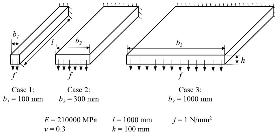
**Fig. 4.8.** Cantilever structures – Presentation of the example for three width/thickness ratios.
