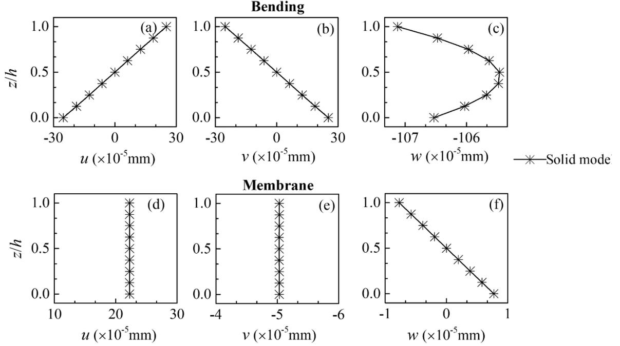
**Fig. 2.1.** Moderately thin square plate under membrane or bending loading – Distribution of through-the-thickness displacements.
