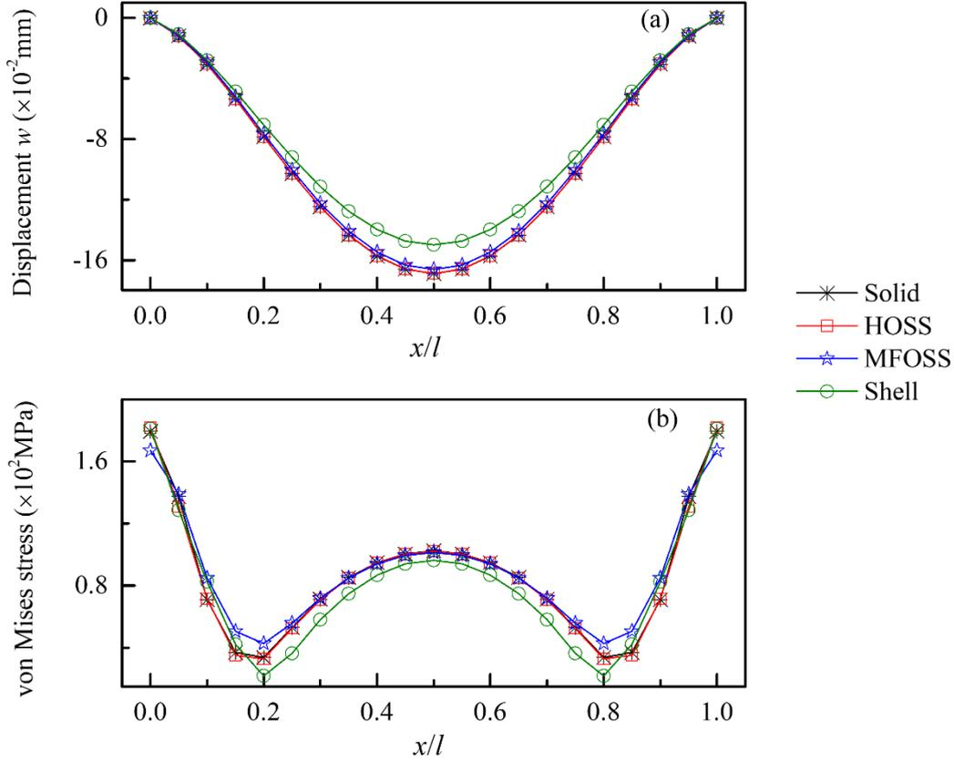
**Fig. 2.16.** Quarter of cylinder under pressure – Distribution of vertical displacement (a) and von Mises stress (b) along a line on the lower face, in the thick case.
