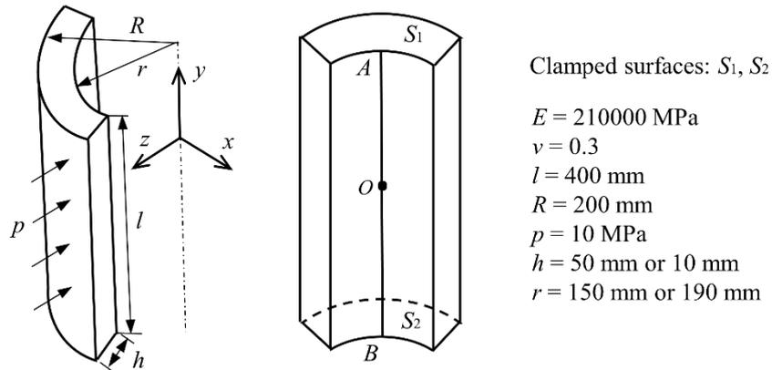
**Fig. 2.12.** Quarter of cylinder under pressure – Presentation of the example.
