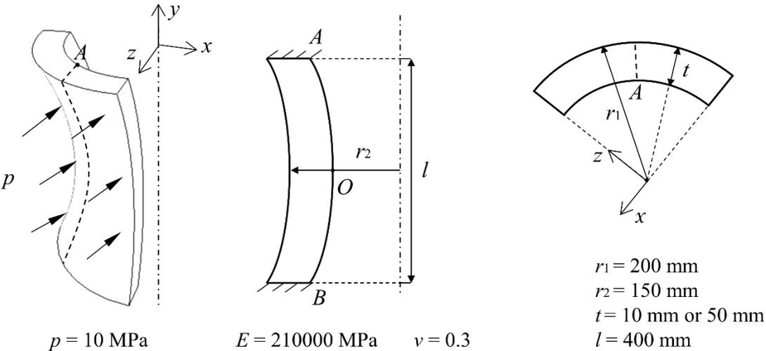
**Fig. 2.17.** Quarter of hyperboloid under pressure – Presentation of the example.
