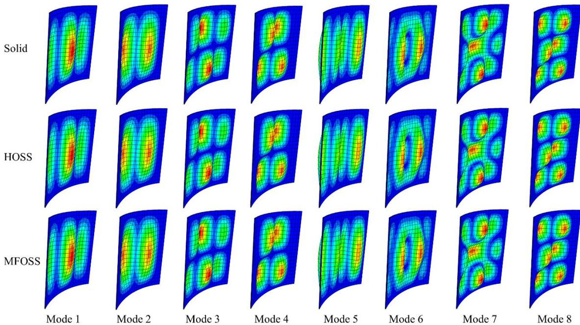
**Fig. 2.28.** Clamped cylindrical panel in free vibration – First eight mode shapes with the reference solid, HOSS, and MFOSS models for the thin case.
