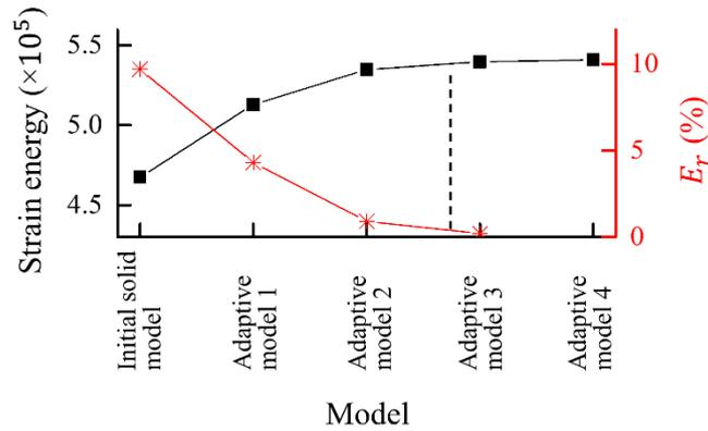
**Fig. 4.18.** “T” shape plates – Convergence of the methodology.
