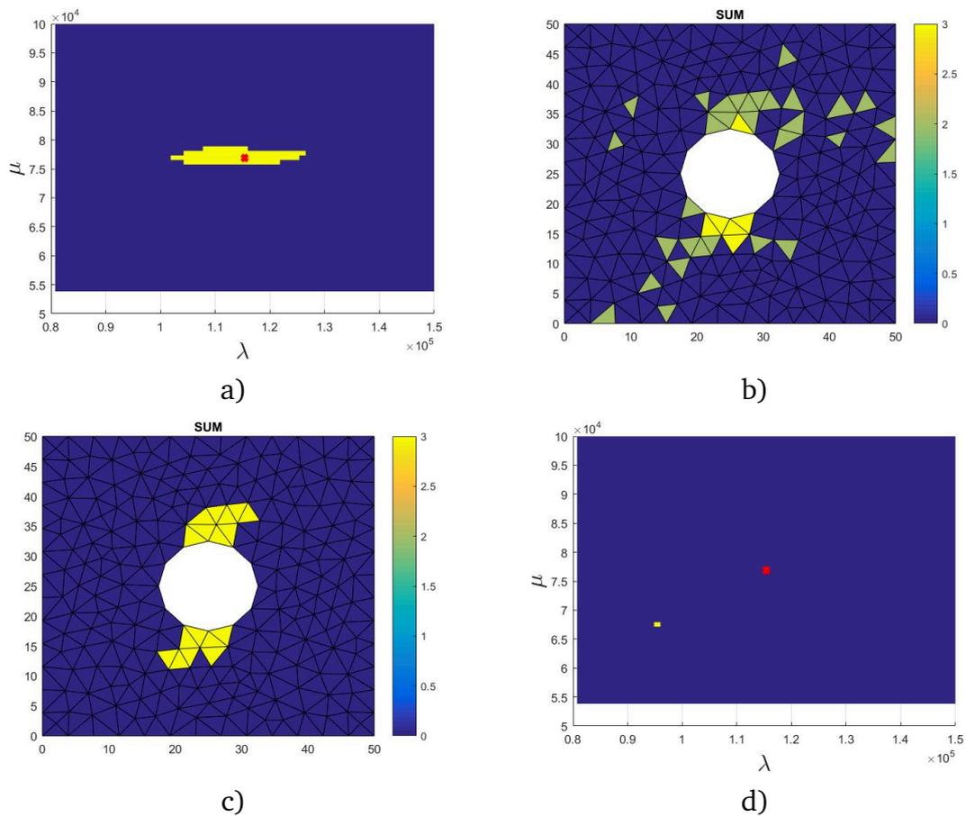
**Figure 4.13** – Damage detection when there is a noise in the data: a) Identification of parameters, b) Location of removed measurements c) approximated damage location, d) identification from the approximated damaged part.
