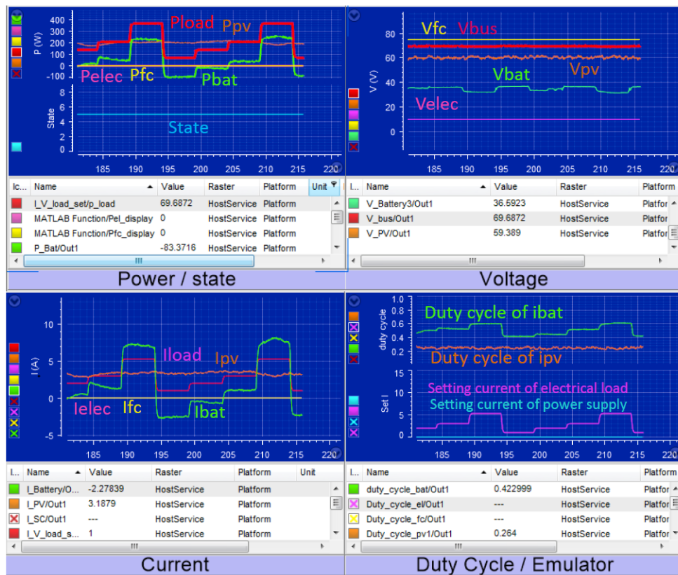
FIGURE 3.9 – Experimental result of rule-based controller in isolated mode
