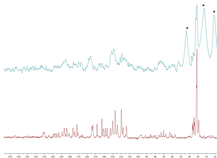
Figure 47: ^{13}\text{C} CP-MAS NMR spectra of Salophen- t Bu-Ni (in red) and Salophen- t Bu-Ni@{NH 2 }-SBA-15 (in blue). The 3 peaks with the asterisk correspond to the {CH 2 } of the propylamine groups of {NH 2 }-SBA-15.
