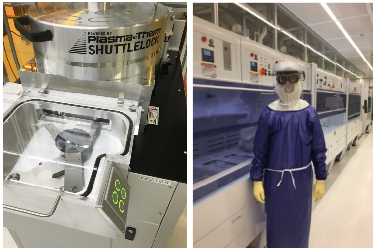
Figure 2.16: Left: A wafer being loaded into an ICP Fluoride etch tool; Right: The author, pictured in Bay 6 of the PNF, wearing protective garments to etch wafers in BHF.
