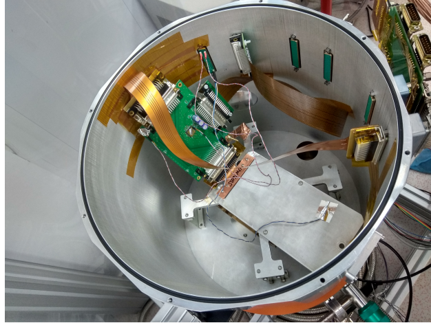
Figure 6.16: CROC chip integration using the LPNHE test system.
