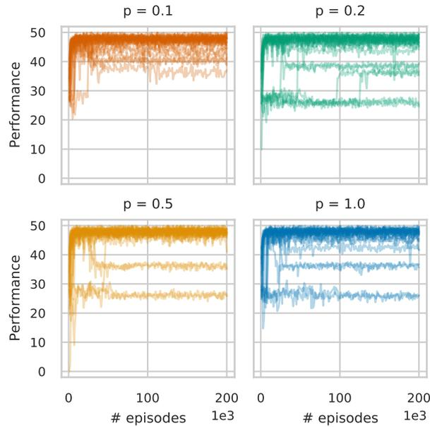
Figure 4.11: Split view of the different performances for different values of  $p$ . Regardless of the value  $p$ , in most of the simulations the agent gets a performance close to the optimal performance at the end of the learning. Like the PPO condition, some simulations reach a sub-optimal equilibrium around 30. Few of them manage to get out of this equilibrium.
