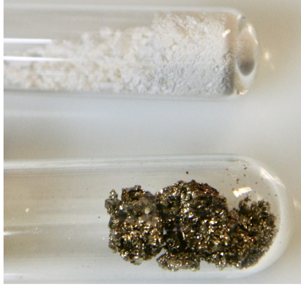
Figure 3.4: Photography of a metallic strontium sample under vacuum (bottom) and open air strontium oxide (top).
