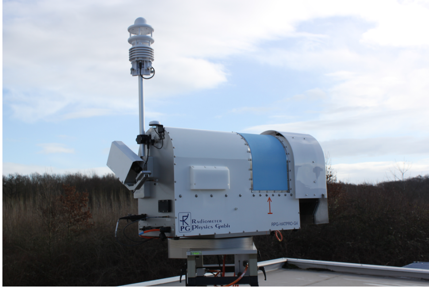
Figure 3.6: A multichannel HATPRO Microwave radiometer.
