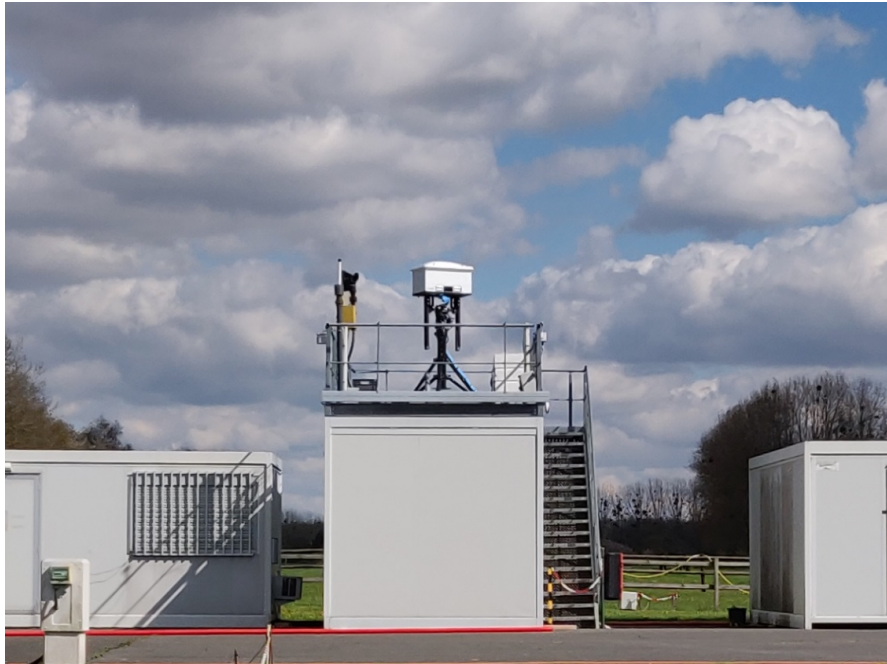
Figure 3.5: A vertically pointing BASTA cloud radar at SIRTa
