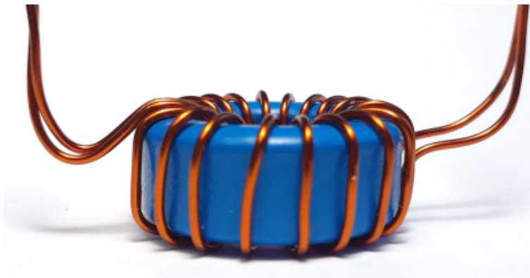
Figure 3.18: Toroidal core with two wound windings-side.
