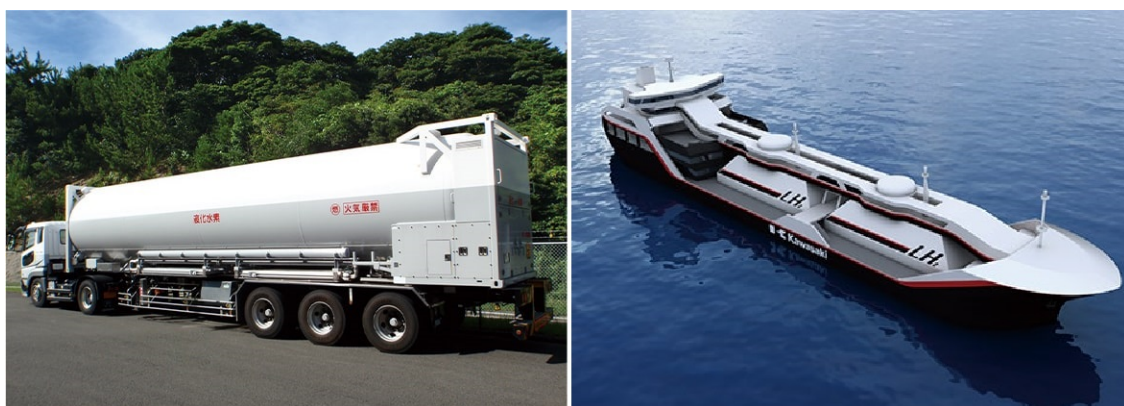
Figure 1.15: Cryogenic trailer and pilot liquefied hydrogen carrier of Kawasaki [101].
