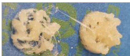
Figure 152. Aspect of the PZQ printlets obtained by directly feeding the physical mixture of praziquantel and PVPVA (1: 1) into the hopper of the 3D printer extruder.
