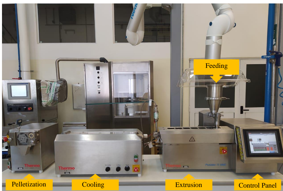
Figure 78. Extrusion system using Pharma 11 extruder.
