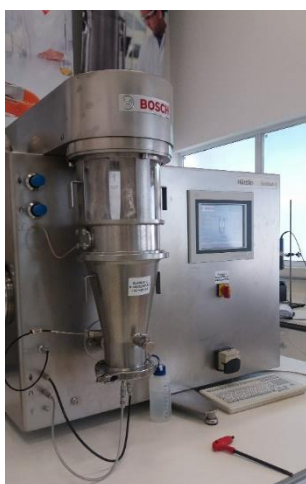
Figure 81. Fluidized bed (Bosh®) for drying the FEXT 1 formulation after granulation.
