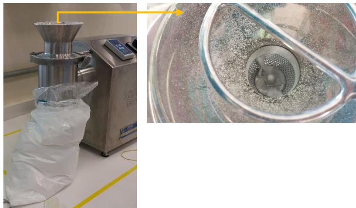
Figure 79. Conical mill (Quadro® Comil® U3 0125) with the respective sieve size used.
