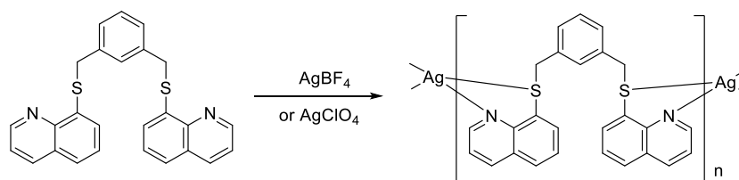
Figure 4-5. Self-assembled helical silver complex with N,S bidentate ligand.
