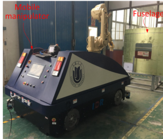
Figure 2.15: Mobile manipulator used for fuselage riveting [Guo et al., 2017]
