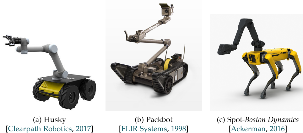
Figure 2.2: Mobile manipulators with different types of locomotion
