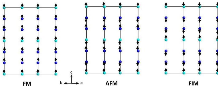
**Figure 5:** Different magnetic configurations of  $Ba_9V_3S_{15}$  used in the DFT+ $U$  calculations.  $V1$  is in light blue and  $V2$  in dark blue, arrows represent spin up ( $\uparrow$ ) and spin down ( $\downarrow$ ).
