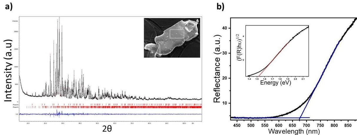
**Figure 2:** (a) Powder XRD Rietveld refinement: the experimental (black) and calculated (red) patterns are superimposed; the difference curve and Bragg positions are represented in blue and red respectively for the main phase (1) and the impurity (2). A SEM image of a single crystal is shown as inset. (b) Diffuse-reflectance spectra and the corresponding Tauc plot as an inset.
