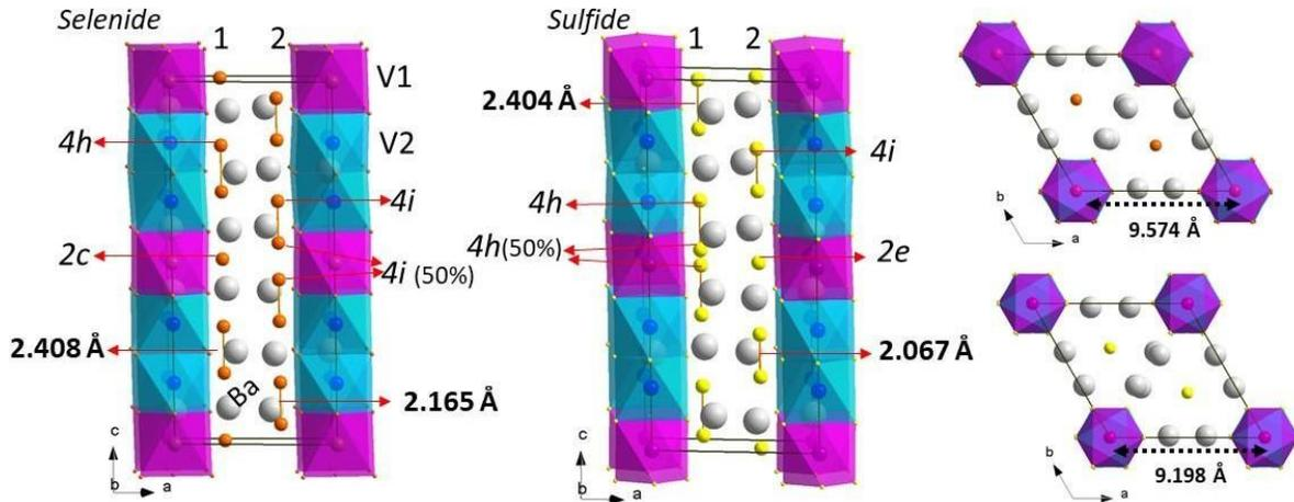
**Figure 3:** Comparison between the title phase and the selenide  $Ba_9V_3Se_{15}$  highlighting the subtle difference of the arrangement within the (di)chalcogenides columns. On the right, projections in the  $ab$  plan showing the distances between two adjacent chains in both phases
