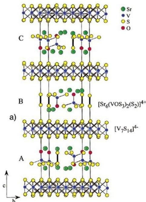
Figure 9. Layered structure of  $Sr_6V_9O_2S_{22}$ <sup>47</sup>
