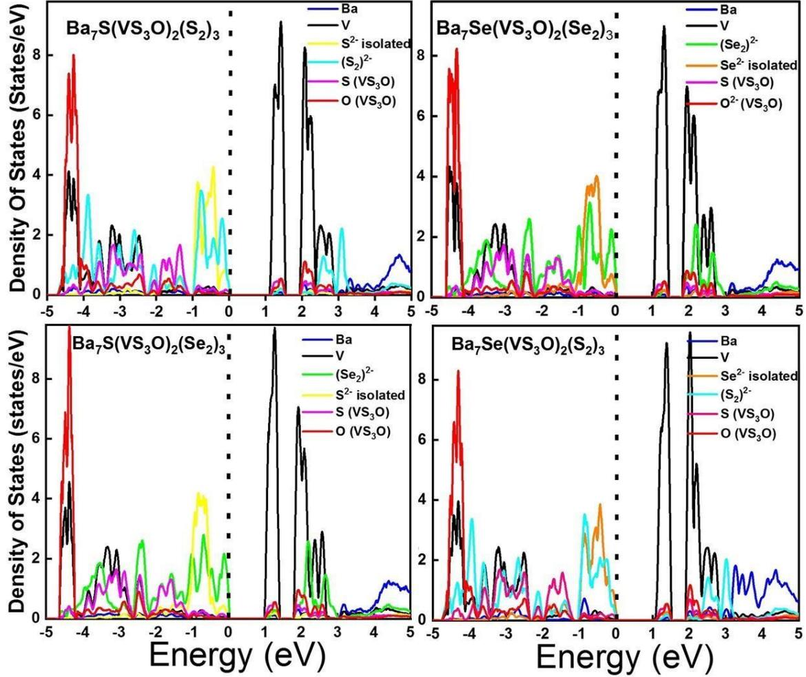
**Figure 6:** Projected Density of States of the four hypothetical phases. The distinct contribution of each species is given: Ba; V, sulfur and oxygen involved in a tetrahedral ( $VO_3S$ ); Q (Q = S, Se) in isolated sites and Q involved in a pair  $Q_2$ .
