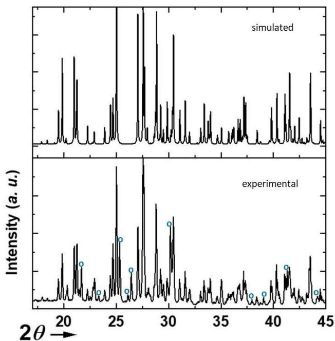
**Figure 1:** X-ray diffraction pattern of  $Ba_5Fe_2In_4ZnS_{15}$  calculated from single crystal refinement, and compared to x-ray experimental pattern of obtained powder, pics impurity are indexed by blue cercles.
