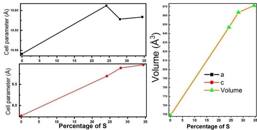
**Figure 2.** Cell parameters and volume evolution with O/S ratio variation for  $Ba_5(VO_{4-\alpha}S_\alpha)Cl$ .
