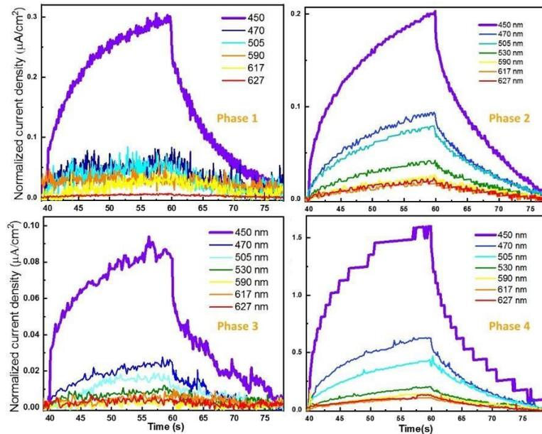
**Figure 7.** Evolution of the transient photo-current response for various wavelengths (performed under a constant luminous flux density of  $42 \text{ mW}\cdot\text{cm}^{-2}$ ) on a film deposited on a ITO/glass substrate.
