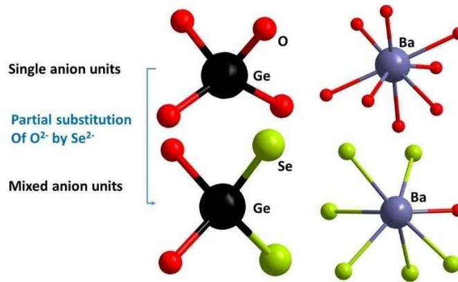
**Figure 3.** BBUs of  $GeO_4$  and  $BaO_7$ ,  $GeO_2Se_2$  and  $BaOSe_6$  polyhedron in  $BaGeO_3$  and  $BaGeSe_2O$ .<sup>14,15</sup>
