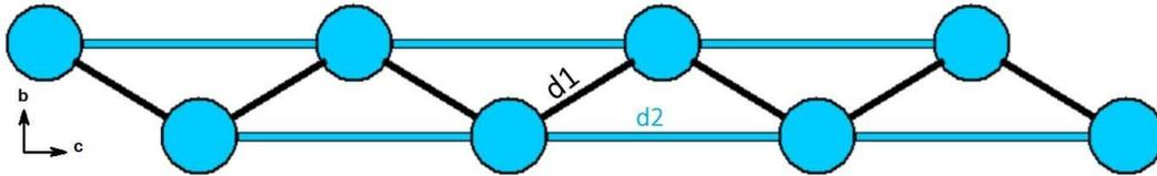
**Figure 6:** Quasi one-dimensional zigzag magnetic chain built from iron atoms in blue with distances of  $J_1$  and  $J_2$  presented in black and blue successively.
