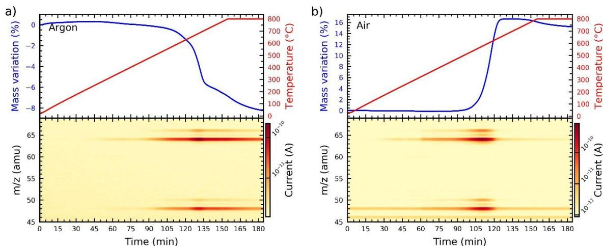
**Figure 4:** Thermogravimetric analysis (upper panes) coupled with mass spectrometry (lower panes) of  $Ba_5(VO_2S_2)_2(S)_2$  a) under argon and b) under synthetic air. The mass variation and the temperature are given as a function of time.
