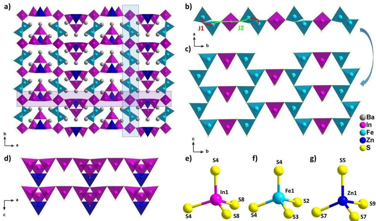
**Figure 2:** a) View of  $Ba_5Fe_2In_4Zn_1S_{15}$  along  $c$  axis b) Magnetic exchange Coupling  $J_1$  and  $J_2$  in the chains extended along  $b$  axis c) interconnection between magnetic chains d) view of lined chains type 2 e) f) g)  $In_1$ ,  $Fe_1$  and  $Zn_1$  coordination respectively.
