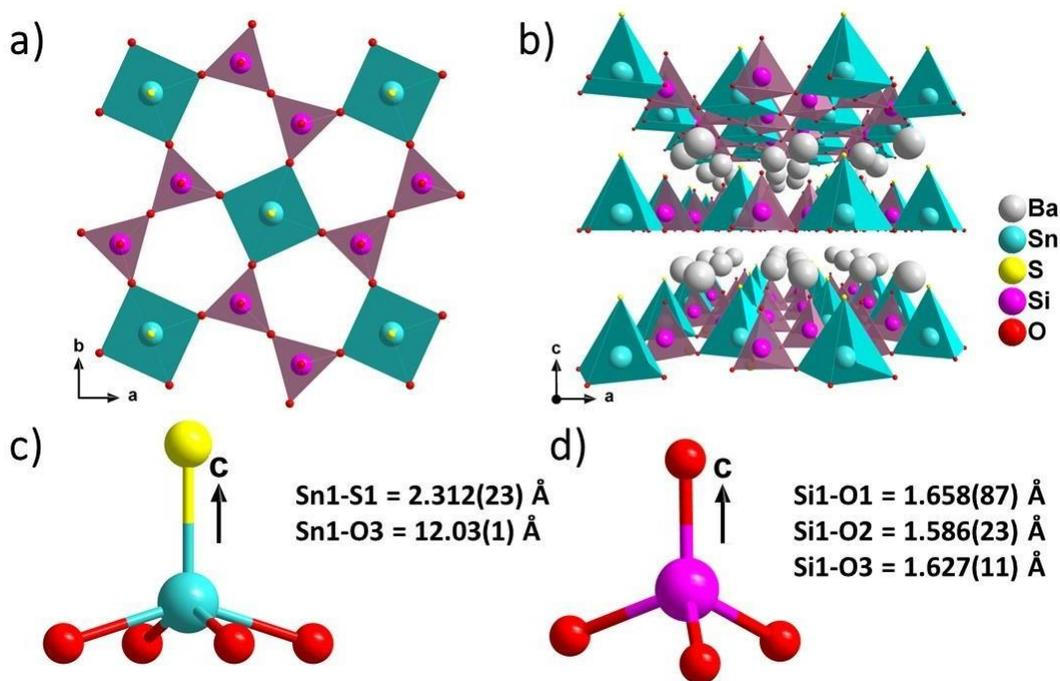
**Figure 4:** (a) Prospection view of a  $\text{SnSSi}_2\text{O}_7$  layer along the  $c$ -axis. (b) A perspective view of  $\text{Ba}_2\text{SnSSi}_2\text{O}_7$  along the  $a$ -axis. (c) The structures of a  $\text{SnO}_4\text{S}$  square pyramid and a  $\text{SiO}_4$  tetrahedron.
