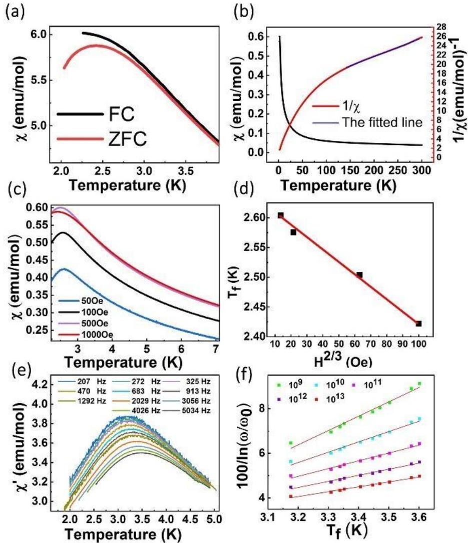
**Figure 4:** a) Inset: zoom of ZFC/FC at low temperature. b) ZFC/FC dc magnetic susceptibility with  $1/\chi$  fitted between 150–300K. c) Isothermal  $M(H)$  at 2 and 300K. d) Evolution of  $T_f$  as a function of the applied magnetic field and the Almeida-Thouless fit as inset. e) Temperature dependence of  $\chi(T)$ . e)  $\chi'(T)$  measured at several fixed frequencies. f) Vogel-Fulcher fit with different fixed  $\omega_0/2\pi$  in the typical range 109–1013Hz for spin-glass.
