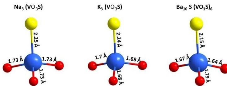
**Figure 6.** Distortion of  $VO_3S$  in  $Na_3(VO_3S)$ ,  $K_3(VO_3S)$ ,  $Ba_{10}S(VO_3S)_6$ .
