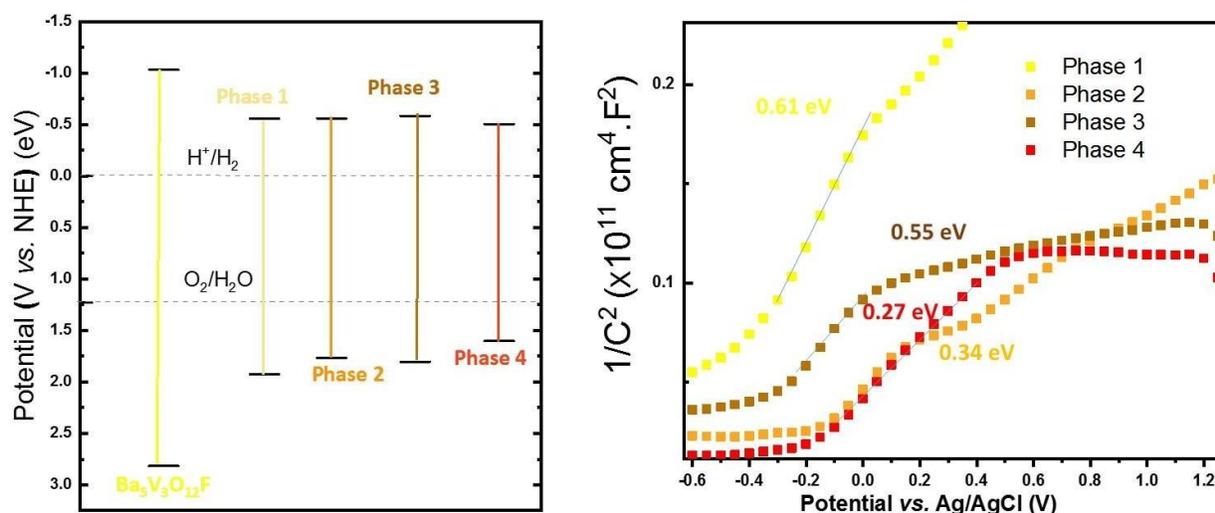
**Figure 6.** a) Calculated band edges positions obtained from empirical calculations for  $Ba_5V_3O_{12}F$  and phases 1,2,3 and 4 respectively. The levels for hydrogen and oxygen evolution are indicated by dashed lines. b) Mott-Schottky plots carried out on the powders deposited on a slide of ITO/glass.
