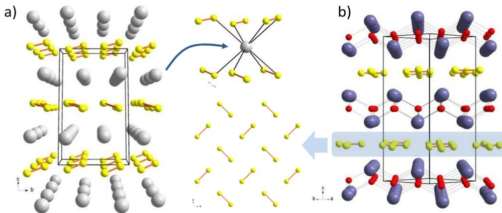
**Figure 3.** a) Structure of  $BaS_2$  with emphasize on Ba environment exhibiting  $d_{Ba-S}$  ranging from  $\sim 3.15$  to  $3.22\text{\AA}$  and b) structure of the phase  $La_2O_2S_2$  with a projection of disulfide layers showing the disulfide pairs 2D arrangement, each ( $S_2$ ) is  $90^\circ$  rotated with respect to its neighbors.
