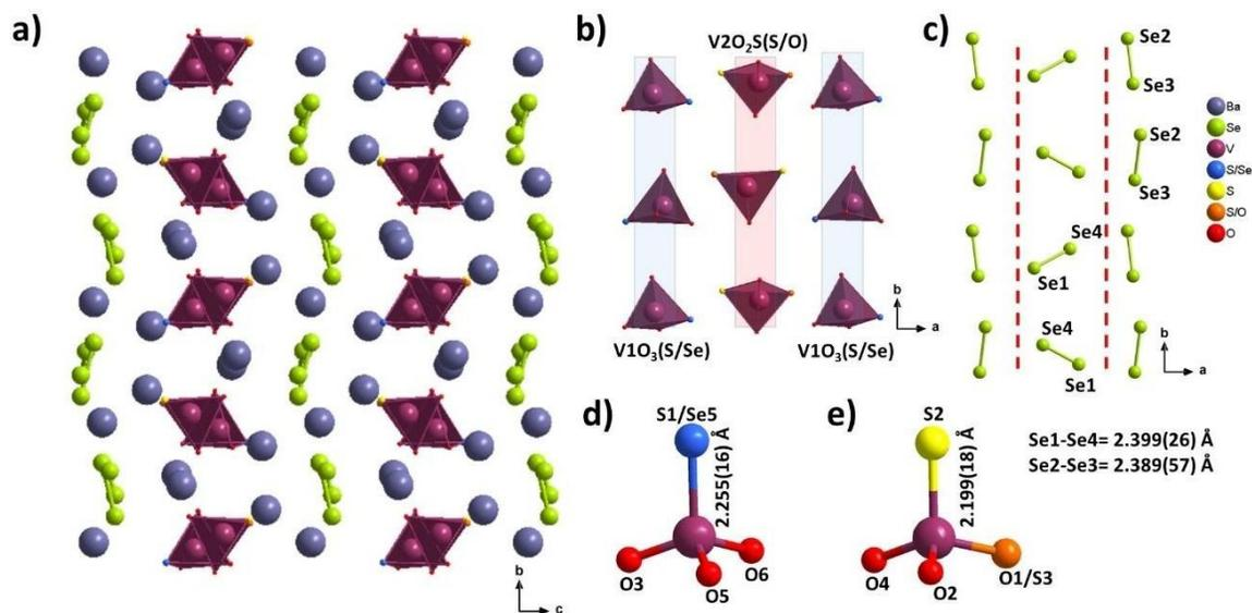
**Figure 1:** (a)  $Ba_5V_2O_{5.29}S_{2.55}Se_{4.16}$  projected along  $a$ -axis (b) Projection of the tetrahedral units along the  $c$ -axis. (c) Slice of the structure showing the  $(Se_2)^{2-}$  pairs along the  $c$ -axis. (d) (e) Slice of the structure showing the tetrahedral  $V1O_3(S/Se)$  and  $V2O_2S(S/O)$  units.
