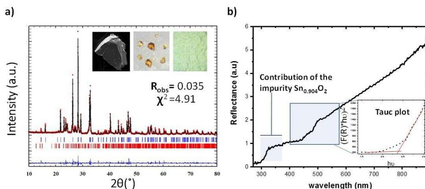
**Figure 5:** (a) Powder XRD Rietveld refinement: the experimental (black) and calculated (red) patterns are superimposed; the difference curve and Bragg positions are represented in blue and red, respectively. A SEM image of a single crystal, a photo of several yellowish crystals and of the powder are also shown as insets. (b) Diffuse-reflectance spectra and the corresponding Tauc plot.
