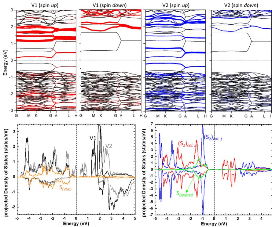
**Figure 4:** Total band structure and fat bands (in red for V1 and blue for V2) (top). Projected density of states (PDOS) of Ba<sub>9</sub>V<sub>3</sub>S<sub>15</sub> (bottom)
