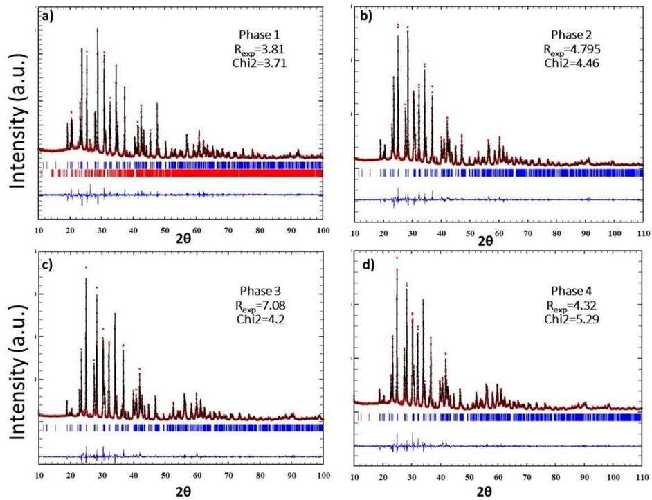
**Figure 1:** a), b), c) and d) Powder XRD Rietveld refinement of Phase 1, 2, 3 and 4 respectively: the experimental (black) and calculated (red) patterns are superimposed; the difference curve and Bragg positions are represented in blue and green respectively.
