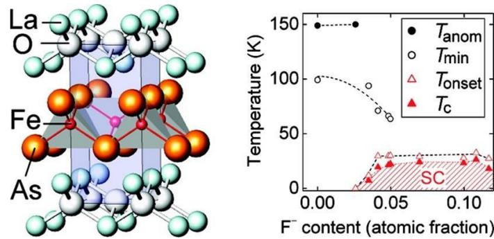
**Figure 2.** crystal structure of LaOFeAs and  $T_c$ ,  $T_{onset}$ , and  $T_{min}$  in the  $\rho$ - $T$  curves as a function of F<sup>-</sup> content ( $x$ ) for La[O<sub>1-x</sub>F<sub>x</sub>]FeAs.  $T_c$  is defined as the temperature where the  $\rho$  value becomes half of that at  $T_{onset}$ .  $T_{anom}$  values for the undoped and LaO<sub>0.97</sub>F<sub>0.03</sub>FeAs are also shown. Dotted curves are guides for eyes. <sup>10</sup>
