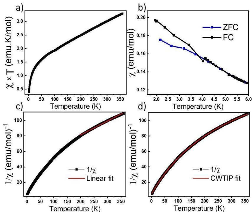
**Figure 3:** a) Temperature dependance of magnetic susceptibility  $\chi \times T$ . b) Zoom of ZFC/FC at low temperature. c) Linear fit of the reciprocal magnetic susceptibility  $1/\chi$  between 200-350K. d) CW TIP fit of the reciprocal magnetic susceptibility  $1/\chi$ .
