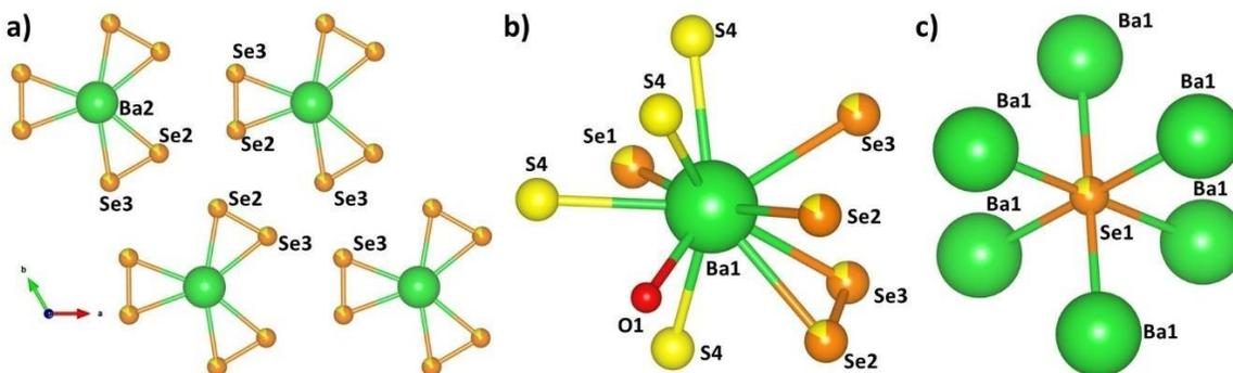
**Figure 3:** a) Se2–Se3 bonds arrangement represented when present in their vicinity: Ba2 and its connectivity with Se2–Se3 bonds. b) Ba1 environments. c) isolated Se1 atom environment. To simplify, the mixed sites Se1/S1 are designed by Se1 and so on for Se2 and Se3.
