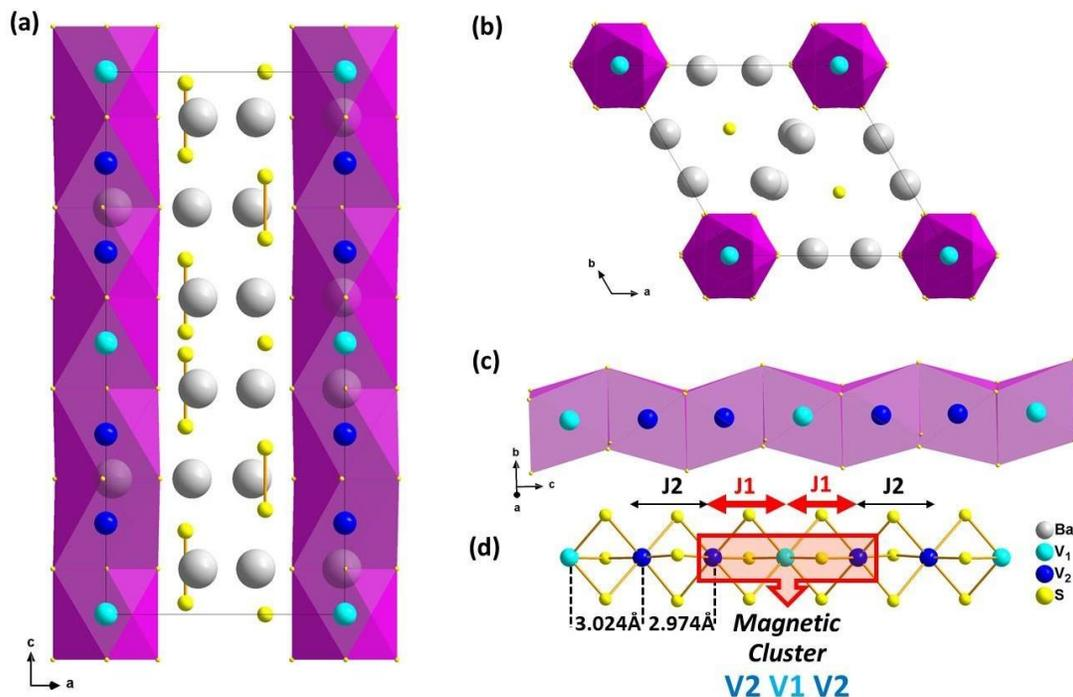
**Figure 1:** a)  $Ba_9V_3S_{15}$  view along  $b$ -axis, b)  $Ba_9V_3S_{15}$  view along  $c$ -axis c)  $VS_6$  based one-dimensional chain d) arrangement of  $V_1$  and  $V_2$  in the spin chain showing strong  $J_1$  (magnetic coupling for  $V_1$ - $V_2$ ) and far weaker  $J_2$  (for  $V_2$ - $V_2$ ) magnetic exchange couplings. This interplay between  $J_1$  and  $J_2$  defines magnetic clusters with the sequence  $(V_2$ - $V_1$ - $V_2$ ).
