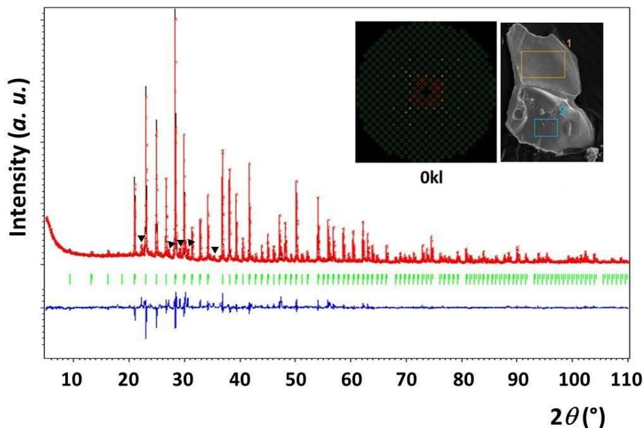
**Figure S2:** XRD Rietveld refinement of a powder of  $Ba_{10}Fe_{7.75}Zn_{5.25}S_{18}Si_3O_{12}$ . The experimental (red) and calculated (black) patterns are superimposed. The difference curve is represented in blue and the Bragg peaks positions in green. The most significant unindexed low intensity impurity peaks are pointed with black triangles. A SEM image of a single crystal and a precession image showing plane  $0kl$  (single crystal XRD) are also shown as insets.
