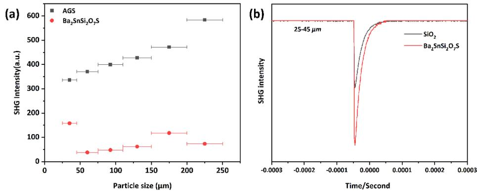
**Figure 7:** (a) Size-dependent SHG responses of Ba<sub>2</sub>SnSi<sub>2</sub>O<sub>7</sub>S and AGS measured with a 2.1  $\mu\text{m}$  incident laser; (b) SHG intensities of Ba<sub>2</sub>SnSi<sub>2</sub>O<sub>7</sub>S and SiO<sub>2</sub> measured by oscilloscope traces of the SHG signals.
