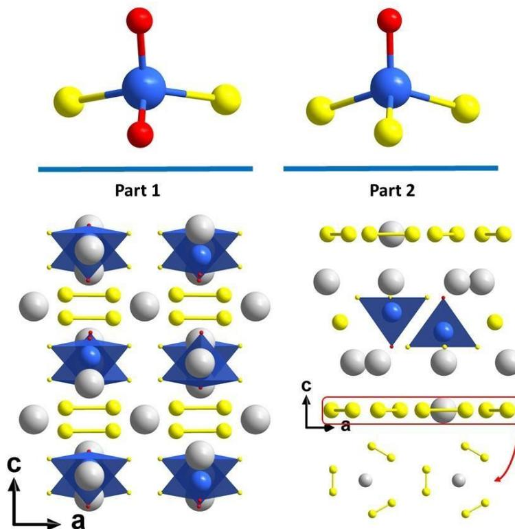
Each phase can be described by two alternating layers: In the first one, at least two anions are surrounding the vanadium cations which form disconnected tetrahedra separated by the large Ba<sup>2+</sup> cation. While the dichalcogenide pairs and the Ba<sup>2+</sup> inserted in the voids constitute the second one. These combined characteristics make the originality of those new compounds.
