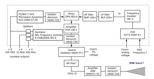
Figure B.8: Electronics rack and channel up to the horn for the micro-wave generation. The dashed line corresponds to components that are not directly accessible as they are in a rack. The components are from Mini-Circuits if not explicitly written. The splitters are power splitters (ZB4PD1-500-S+, ZB4CS-700-10W-N). The BP filter and MW horn are detailed in the main text.
