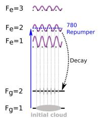
Figure E.2: Subwavelength imaging principle where a 780 repumper laser is used. The blue dashed line represents the resonant position of the 780 laser. The ground state  $|g\rangle$  refers to  $5S_{1/2}$  and the excited state  $|e\rangle$  to  $5P_{3/2}$ .
