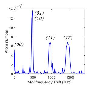
Figure B.12: MW spectroscopy of the molasses without optical pumping but with a BMF of compliance equal to 4V. The MW pulse is 300 µs and the MOT loading time is 500 ms. The MW pulse is done in situ and the atom number is measured along ccd45 axis after TOF=15ms.
