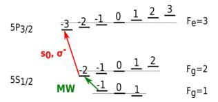
Figure D.5: D<sub>2</sub>-line of <sup>87</sup>Rb atomic structure where atoms are transferred with a MW transition to  $|F_g = 2, m_F = -2\rangle$  and imaged on the cycling transition using a  $\sigma$ -polarized light.
