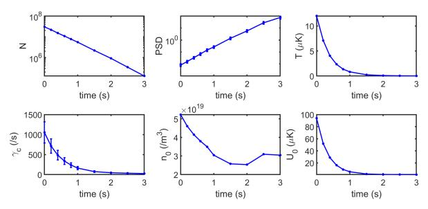
Figure B.29: Atom number, phase-space density, temperature, two-body collision rate, central density and trap depth as a function of the evaporation time using classical gas thermodynamics.
