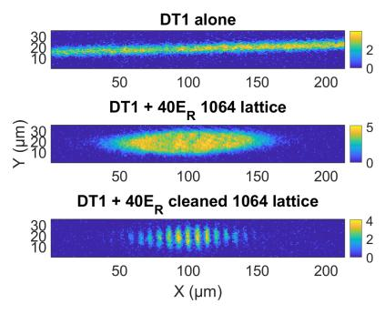
Figure F.8: Raw images of in situ optical densities for DT1 alone with no trapping along the longitudinal axis, DT1+40 $E_r$  1064 lattice imaging on resonance and DT1+40 $E_r$  1064 lattice which has been cleaned (steps  $t_1$ ,  $t_2$ ,  $t_4$ ) using the 1529 lattice then imaged on resonance on the cycling transition without 1529 nm beams.
