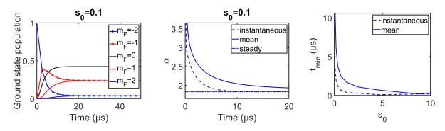
Figure C.13: Case of  $\pi$ -polarized light and  $(\rho_{-2-2}^{(0)}, \rho_{-1-1}^{(0)}, \rho_{00}^{(0)}, \rho_{11}^{(0)}, \rho_{22}^{(0)}) = (1, 0, 0, 0, 0)$ : ground state population dynamics, instantaneous and mean value of  $\alpha$  and minimum pulse duration to reach 90% of the steady-state value.
