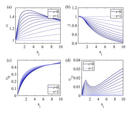
Figure C.8: Model parameters a)  $\alpha$ , b)  $\beta$ , c)  $\eta_0$  and d)  $\eta_{\infty}$  as a function of the incoherent intensity  $s_i$  for polarization degrees  $r \in [0, 1]$  by step of 0.1. The shaded area represents the 95% confidence interval of the fits and is very small on the plots. In c), the limit cases r = 0 and r = 1 exactly coincide with the analytical solutions given in Eq. (C.54) and the second term of Eq. (D.31) respectively.
