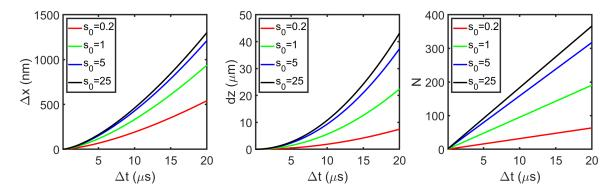
Figure D.2: Random walk displacement in the transverse plane  $\Delta x$ , longitudinal displacement along the beam propagation dz and scattering number N vs. the probe durations for many saturation parameters. We have  $DOF = 22 \ \mu m \ (NA = 0.185)$  and  $t_{pix} = 848 \ nm$ .
