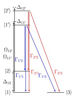
Figure C.15: A 5-level atom with one more excited state and one more ground state compared to the 3-level system.
