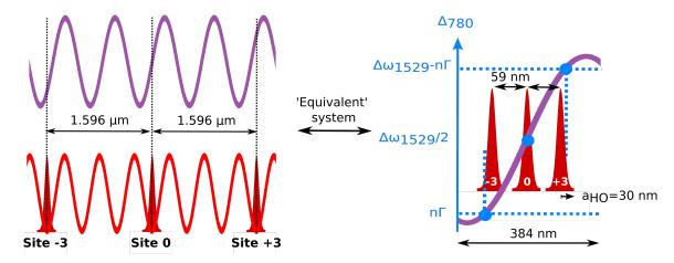
Figure F.10: Atomic densities in sites 0,  $\pm 3$  which are 1.596 µm apart from each other and the equivalent system where two sites would be at 59 nm from each other.
