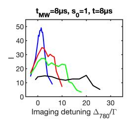
Figure III.3: BAT curve example of a dataset showing the integrated transmission as a function of the imaging beam detuning for different light shifts on  $|F_e = 3, m_F = -3\rangle$ . Each point has been average over 2 runs. The curves from top to bottom correspond to powers per beam of: 0.58, 1.74, 2.9 and 5.8 mW.
