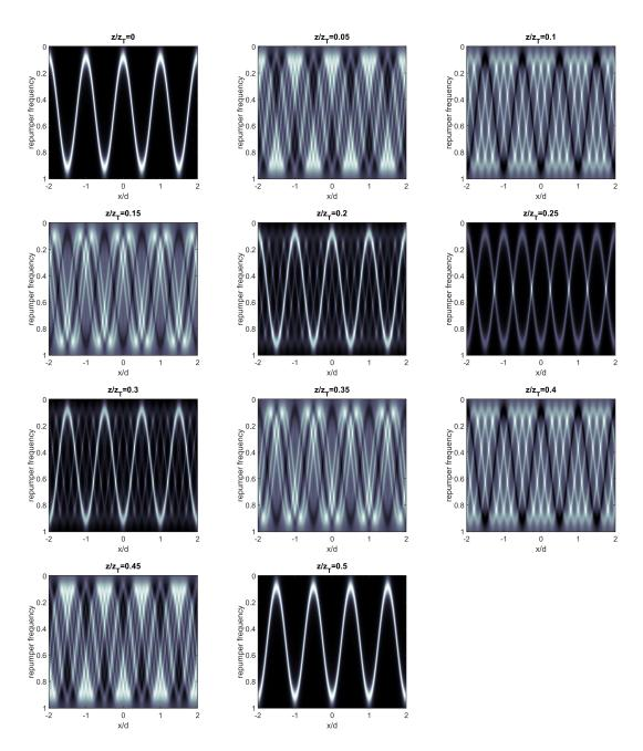
Figure III.2: Simulations of the tomography images at different propagation distances for the co-propagating 1529 nm beams with d=8 µm, t=10 µs,  $s_0$ =0.15 and a light shift of  $17\Gamma$ .
