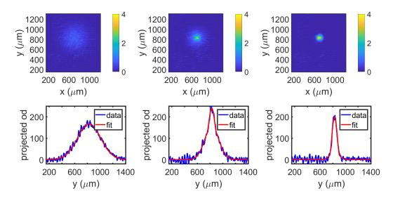
Figure B.31: Optical density after the evaporation by lowering the magnetic gradient while the atoms are loaded in the crossed dipole trap (DT1+DT2). Projections along y-axis are the data and the 2D fit with a bi-modal distribution.
