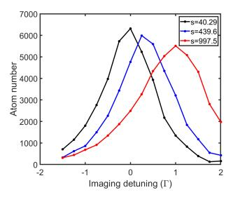
Figure IV.8: Atom number as a function of the imaging detuning (cooler transition) for different lattice trap depths measured in situ.
