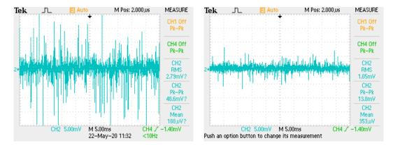
Figure II.1: Voltage noise from the Dev3 ao3 passing through the BNC2110 connector block (left) or by-passing it (right). It is measured with an oscilloscope TBS1064 (DC-60 MHz).
