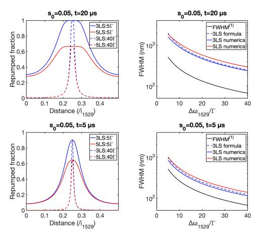
Figure E.8: Repumped fraction and FWHM for the repumper detuning tuned at the middle of the modulation of  $F_e = 2$  as a function of the light shift of  $F_e = 2$ . The modulation interfringe is 8.3 µm. We show them for a pulse duration of 5 µs and 20 µs.
