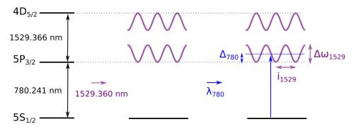
Figure E.1: Subwavelength imaging principle: a 1529 optical lattice intensity dresses the  $5P_{3/2}$  state and a 780 probe is resonant only with certain positions.
