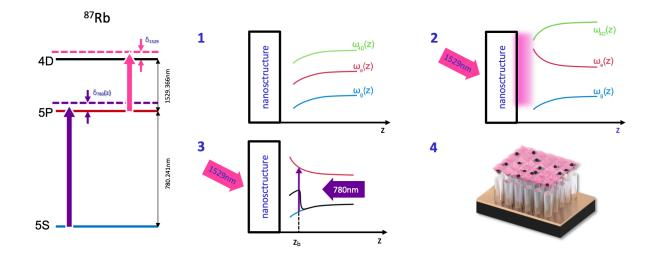
Figure A.4: Method from (Bellouvet et al., 2018) to generate near-field traps. 1) Casimir-Polder forces dress the atom in close vicinity to the surface, 2) A strong laser intensity at 1529 nm generates an evanescent wave dressing the first excited state, 3) A 780 nm laser couples the ground state and the excited state to form a barrier at position  $z_b$ , 4) Structuring the surface modulates Casimir-Polder forces and generates a subwavelength lattice with the periodicity of the nanostructure.
