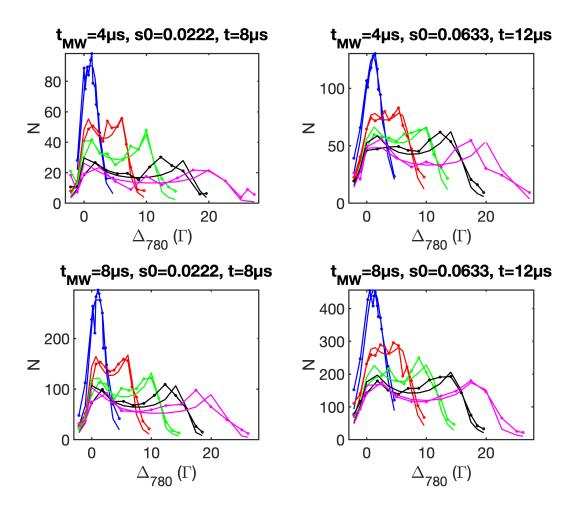
Figure E.17: BAT curves for the co-propagating case: number of atoms integrated in 1 interfringe vs. the repumper detuning. Within a plot, the curves from top to bottom correspond to powers per beam of: 0.29, 0.87, 1.45, 2.03 and 2.9 mW.
