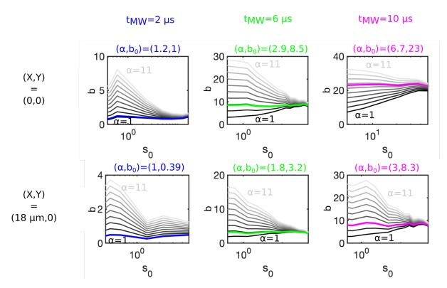
Figure D.11: Cross-section calibrations curves for  $t_{MW}=2$  µs,  $t_{MW}=6$  µs and  $t_{MW}=10$  µs at two positions in the cloud. Black curves correspond to different values of  $\alpha$ . The colored curve is the one which has the value of  $\alpha$  which minimizes std(b) with the corresponding values of  $\alpha$  and b in the plot title.
