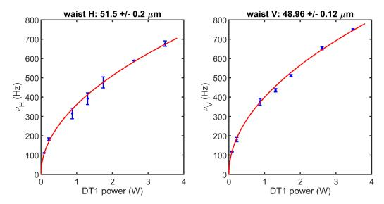
Figure B.28: Trap frequency of DT1 in a hybrid trap for a magnetic gradient of 29 G/cm, TOF=12 ms, trap depth compression pulse of 150 µs at 4V. All frequencies are measured with 'imaging along DT1'. Errorbars are fit errors.
