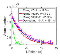
Figure B.5: MOT lifetime during a burst event, during the rise and the fall of the peak. Points are data from 26/09/2019 and solid lines are exponential fits of the type  $ae^{-t/\tau} + b$ .
