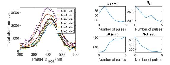
Figure F.12: Total atom number after lattice cleaning with N=0 and M repumper pulses vs. the piezo displacement. Lattice depth is  $1000E_r$  and the light shift is 106 MHz. Black solid lines are fits with Eq. (F.11).
