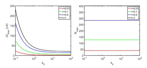
Figure D.3: Doppler condition on the maximum pulse duration and maximum scattering number vs. the saturation for different parameter r.
