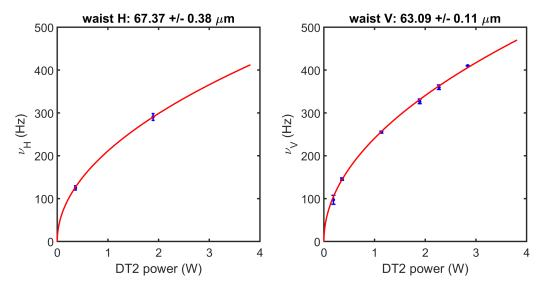
Figure B.27: Trap frequency of DT2 in a hybrid trap for a magnetic gradient of  $29~\mathrm{G/cm}$ , TOF=12 ms, trap depth compression pulse of 150 µs at 6V. The vertical frequency is measured with 'imaging along DT1' and the horizontal frequency is measured with 'ccd45' imaging axis. Errorbars are fit errors.
