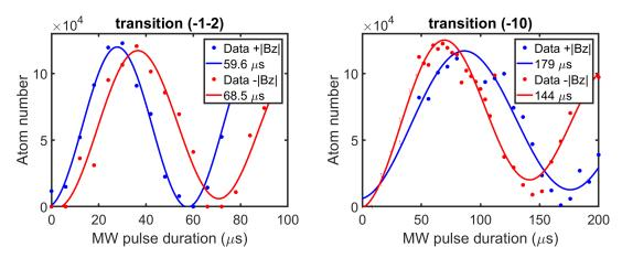
Figure B.33: Rabi oscillation data with their fits with a damped sine function for the two transitions  $|F_g=1,m_F=-1\rangle$  to  $|F_g=2,m_F=-2\rangle$  and  $|F_g=1,m_F=-1\rangle$  to  $|F_g=2,m_F=0\rangle$ . The fit function is a sine function with an exponential damping which takes decoherence into account.
