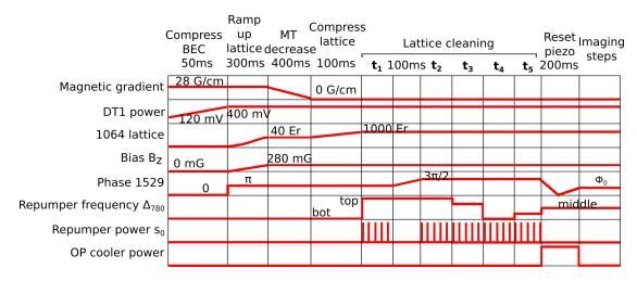
Figure F.7: Experimental sequence for the cleaning stage in the 1064 lattice.
