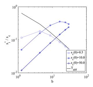
Figure D.16: Forwards incoherent transmission vs. the optical density for three initial coherent saturations (blue lines). The black line is the diffuse transmission given by  $T_{diff} = \frac{1+0.7104}{b+2\times0.7104}$  (Guerin, Rouabah, and Kaiser, 2017).
