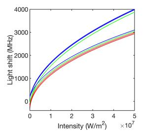
Figure E.5: Light shifts at the laser frequency of 1529.36098 nm for all states of F = 0 (black), F = 1 (red), F = 2 (green) and F = 3 (blue) of  $5P_{3/2}$  vs. the 1529 intensity. All curves start at their hyperfine shift at zero intensity and referred to the fine structure energy. The black curve is at the bottom, very close to the first red curve.
