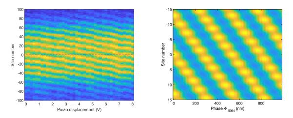
Figure F.6: Integrated repumped atom numbers vs. piezo displacement: experiment (left) and theory (right). The horizontal black dashed line is a guide for the eye to follow site 0. We use the right plot to calibrate the piezo displacement of the left plot.
