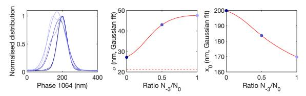
Figure F.14: (left) Dashed lines are the expected repumped population and solid lines are Gaussian fits; Gaussian (middle) width  $\sigma$  and (right) central position  $x_0$  of the Gaussian fits for different initial population ratio (0, 0.5 and 1) in sites 0 and -3. Population in site +3 is always 0. The red dashed line is the harmonic oscillator atomic density width  $\sigma_0$ .
