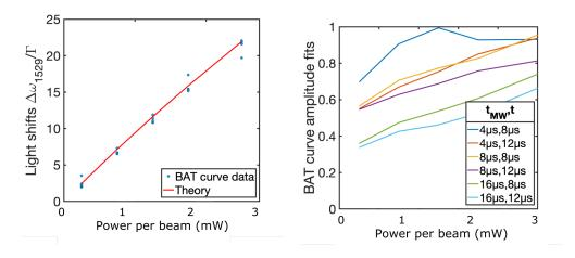
Figure E.18: The two fit parameters from the BAT curves in the co-propagating case with  $i_{1529} = 8.3 \, \mu \text{m}$ . Left: total light shift amplitude  $c_2$  extracted from the fit (blue circles) and the expected theoretical light shift (red). Right: atom number scaling factor  $c_1$ .
