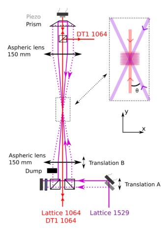
Figure F.5: Double lattice at 1064 and 1529 that can be realized on the experiment. All beams can be seen on the main experimental setup of Fig. B.2.
