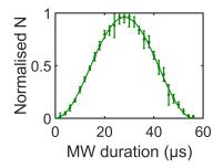
Figure D.6: Rabi oscillation of the normalized atom number (points) between  $|F_g=1,m_F=-1\rangle$  and  $|F_g=2,m_F=-2\rangle$  as a function of the MW duration and a sinusoidal fit (solid line). The data are normalized with an optically repumped total atom number.
