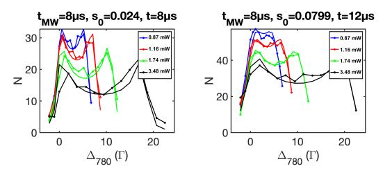
Figure E.20: BAT curves for the counter-propagating case: number of atoms integrated in 1 interfringe vs. the repumper detuning. The legend corresponds to the 1529 power setpoint with a conversion factor for the power per beam of 0.58 mW/V. Solid lines with points are experimental data and pure solid lines are fits using a 3LS model for the repumped fraction with two free parameters: a light shift and an atom number amplitude factor.
