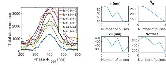
Figure F.13: Total atom number after lattice cleaning with N=M repumper pulses vs. the piezo displacement. Lattice depth is  $1000E_r$  and the light shift is 106 MHz. Black solid lines are fits with Eq. (F.11).
