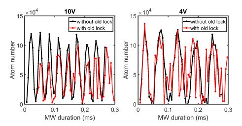
Figure B.9: Rabi oscillations when transferring atoms from  $|F_g=1, m_F=-1\rangle$  to  $|F_g=2, m_F=-2\rangle$ . The atom number is measured with the imaging axis along the MOT at TOF=15 ms, and for a BEC in a crossed dipole trap with a bias magnetic field along z of about 280 mG. We made sure that the MW frequency was resonant with the atoms by scanning the MW frequency and finding the peak value.
