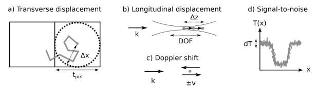
Figure D.1: a) Transverse displacement due to atom random walks compared to a camera pixel size, b) longitudinal displacement along the depth-of-field of the microscope after scattering events, c) Doppler shifts due to scattering and d) signal-to-noise amplitude of the transmission.
