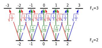
Figure C.1: The closed transition  $|F_g=2\rangle$  to  $|F_e=3\rangle$  for the  $D_2$ -line of <sup>87</sup>Rb with the Clebsch-Gordan couplings of  $\pi$  and  $\sigma_{\pm}$  transitions.
