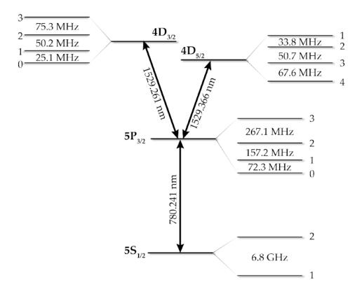
Figure I.1: Atomic structure of a few levels of <sup>87</sup>Rb from (Bellouvet, 2018).
