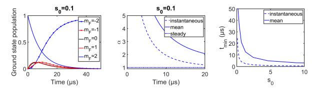
Figure C.10: Case of  $\sigma^-$ -polarized light and  $(\rho_{-2-2}^{(0)}, \rho_{-1-1}^{(0)}, \rho_{00}^{(0)}, \rho_{11}^{(0)}, \rho_{22}^{(0)}) = (0, 0, 0, 0, 1)$ : ground state population dynamics, instantaneous and mean value of  $\alpha$  and minimum pulse duration to reach 90% of the steady-state value.
