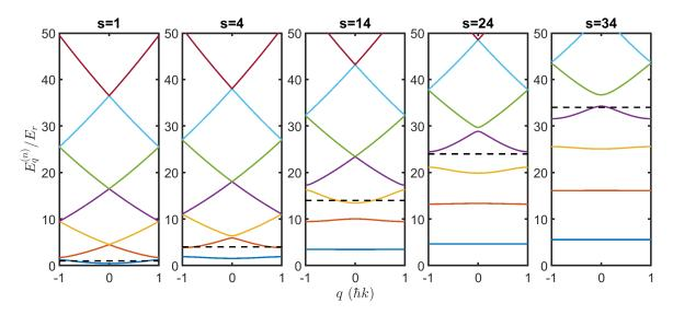
Figure A.1: Band structure from bands n=0 to n=6 for many trap depths s. The dashed black lines are the lattice depth levels.
