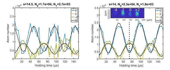
Figure IV.5: Kapitza-Dirac oscillations after an expansion of 5.9 ms for the same power setpoint but with the same diffraction order for DT1 and lattice AOMs (left), or different AOM diffraction orders (right). The solid black line is a global fit on momentums  $0, \pm 2\hbar k$ . Each data point is a single run.
