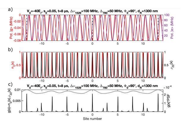
Figure F.3: a) Ground and excited state lattice potentials for  $\theta = 5.7^{\circ}$ , b) periodic lattice atomic density  $n_0(x)$ , repumped population  $\rho_{22}(x)$  and c) g(x) (black solid line) and image after applying the microscope point spread function g(x) \* PSF(x) (black dashed line) for s = -40 and  $\Phi_0 = 90^{\circ}$ .
