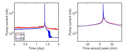
Figure B.4: Ionic pump current around a burst peak and zoom around the main peak. IP1 and IP2 refer to the two ionic pumps: 1 for near 2DMOT and 2 for far from 2DMOT. The conversion factor from the ionic current  $P_{nA}$  in nA to the actual pressure in mbar is  $P_{mbar} = 1.33 \times 10^{-10} P_{nA}$ .
