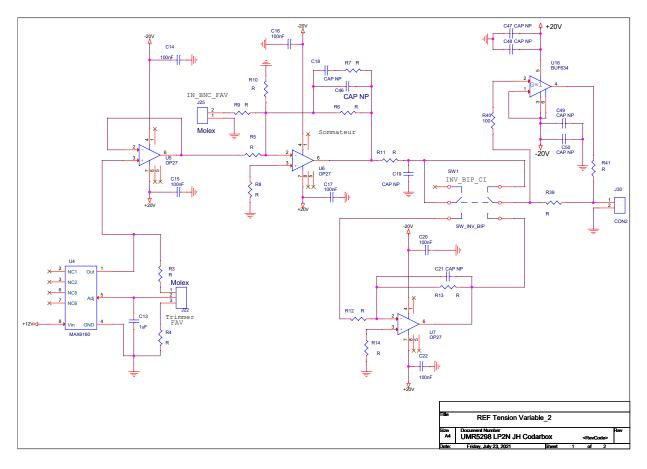
Figure II.5: Main electronics circuit for the reference voltage racks.
