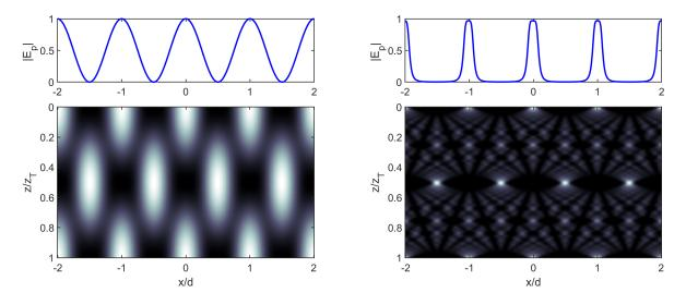
Figure III.1: 1D plots of the probe transmission ( $|E_p| = |A|$ ) for a sinusoidal (left) and square (right) grating at z = 0 and 2D plots of the Talbot carpets.
