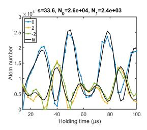
Figure IV.6: Kapitza-Dirac oscillations after an expansion of 5.9 ms for a trap depth of 33.6. The solid black line is a global fit on momentums  $0, \pm 2\hbar k$ . Each data point is a single run.
