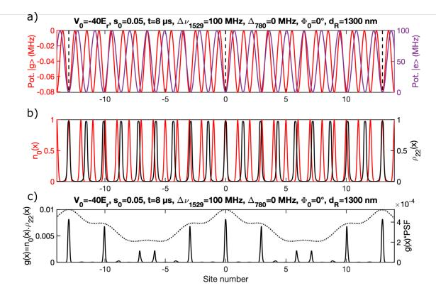
Figure F.1: a) Ground and excited state lattice potentials for  $\theta = 5.7^{\circ}$ , b) periodic lattice atomic density  $n_0(x)$ , repumped population  $\rho_{22}(x)$  and c) g(x) (black solid line) and image after applying the microscope point spread function g(x) \* PSF(x) (black dashed line) for s = -40 and  $\Phi_0 = 0^{\circ}$ .
