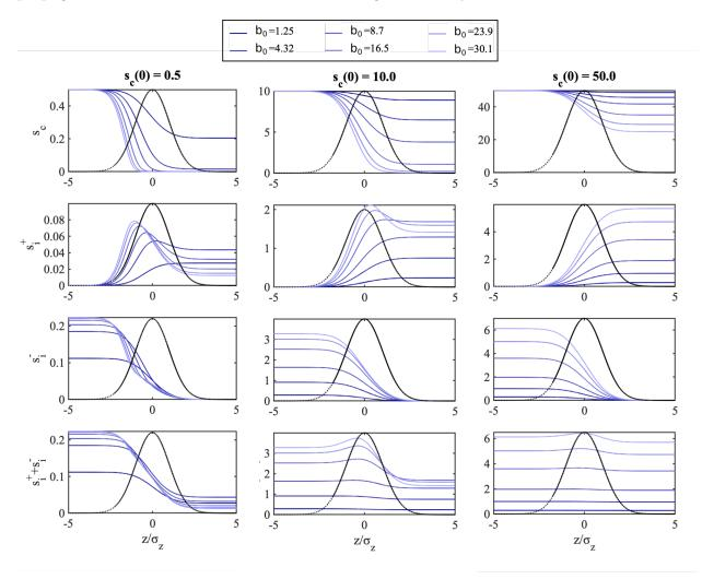
Figure D.14: Saturation profiles for the coherent  $s_c(z)$  and incoherent parts  $s_i^+(z)$ ,  $s_i^-(z)$  and  $s_i^+(z)+s_i^-(z)$ , for coherent input saturations of  $s_c(0)=0.5, 10, 50$  and optical densities  $b_0$  from 1.25 (dark blue solid line) to 30.1 (light blue solid line). The black dotted line is the Gaussian atomic density profile with an arbitrary amplitude to match the plot size. The x-axis is normalized by the Gaussian width  $\sigma_z = 5 \,\mu\text{m}$ .
