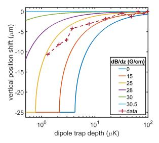
Figure B.32: Expected gravity sag in our hybrid trap potential with DT1 (waist of 50 μm) compared to a single run dataset.
