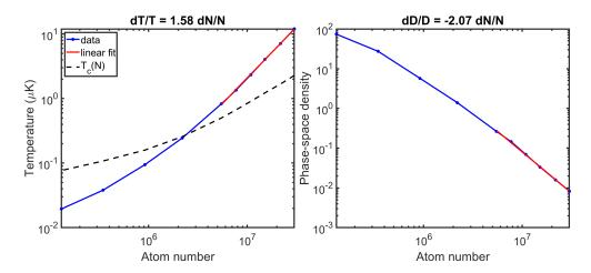
Figure B.30: Forced evaporation in the hybrid trap with a single dipole trap (DT2): data (blue) and linear fit (red). The linear fit parameters are for the temperature  $\alpha = 1.58$  and for the phase-space density -2.07.
