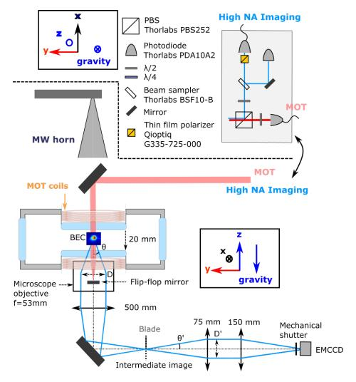
Figure B.18: Schematics of the high NA imaging axis.
