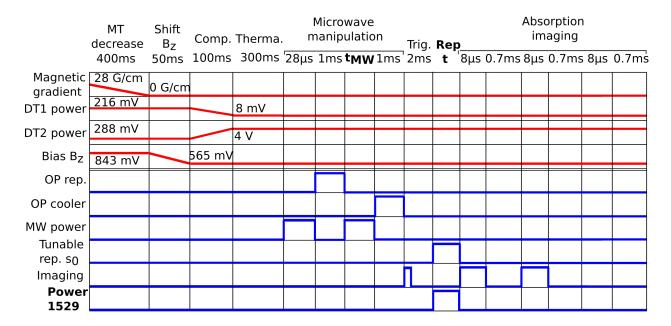
Figure E.16: Experimental sequence for evaluating subwavelength resolutions on the repumper transition. In red are analog channels and in blue TTL channels.
