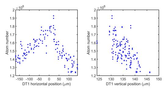
Figure B.25: Scan of the mirror horizontality. The 0 on the x-axis is referenced to the in situ position of the magnetic trap.
