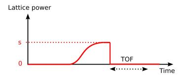
Figure IV.1: Ramp diagram of the adiabatic loading of the BEC in the 1D lattice followed by a time-of-flight after suddenly switching off the lattice light.
