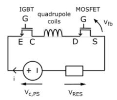
Figure II.4: Electronic circuit for quadrupole coils current feedback.
