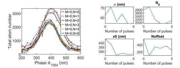
Figure F.11: Total atom number after lattice cleaning with M=0 and N repumper pulses vs. the piezo displacement. Lattice depth is  $1000E_r$  and the light shift is 106 MHz. Black solid lines are fits with Eq. (F.11).
