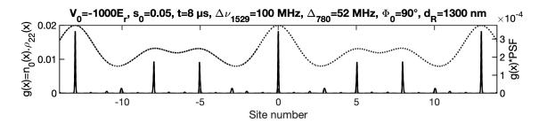
Figure F.4: Repumped population g(x) (black solid line) and image after applying the microscope point spread function g(x)\*PSF(x) (black dashed line) for s=-1000 and  $\Phi_0=90^\circ$ . It compares to Fig. F.3.
