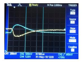
Figure B.20: Transient time evolution of the turn on of the current (blue) giving a constant magnetic field (yellow) window over 500 µs after a rising time of 250 µs.
