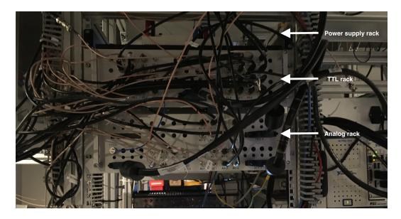
Figure II.2: Picture of the new system with buffers for distributing the voltages on the experiment.
