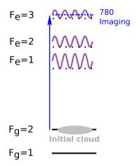
Figure E.3: Subwavelength imaging principle where a 780 imaging laser is used. The blue dashed line represents the resonant frequency of the 780 laser. The ground state  $|g\rangle$  refers to  $5S_{1/2}$  and the excited state  $|e\rangle$  to  $5P_{3/2}$ .
