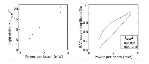
Figure E.21: The 2 fit parameters from the BAT curves in the counter-propagating case with  $i_{1529} = 8.3 \,\mu\text{m}$ . Left: total light shift amplitude extracted from the fit (blue circles). Right: atom number scaling factor.
