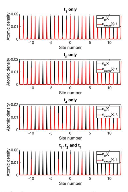
Figure F.9: Independent coarse cleaning steps corresponding to  $t_1$ ,  $t_2$  and  $t_4$ . In black is the lattice with equal initial population for all sites and red is the remaining population after a given cleaning step indicated in each subplot title.
