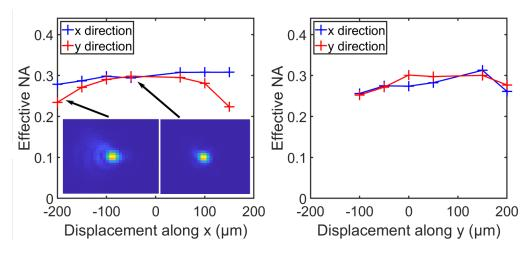
Figure B.16: Characterization using a 1  $\mu$ m pinhole: NA extracted from a fit with a 2D Gaussian convolved with the 1  $\mu$ m pinhole as a function of the sample displacement along x and y around the best minimum spot size. The images show raw data of the measured PSF where come aberrations can be seen.
