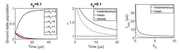
Figure C.9: Case of  $\sigma^-$ -polarized light and  $(\rho_{-2-2}^{(0)}, \rho_{-1-1}^{(0)}, \rho_{00}^{(0)}, \rho_{11}^{(0)}, \rho_{22}^{(0)}) = (0.2, 0.2, 0.2, 0.2, 0.2)$ : ground state population dynamics, instantaneous and mean value of  $\alpha$  and minimum pulse duration to reach 90% of the steady-state value.
