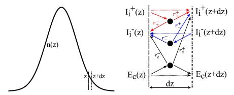
Figure D.13: 1D model for the coherent and incoherent propagation and conversion of light between adjacent layers. The coherent and incoherent scattering rates are given by Eq. (D.31). The spatial repartition are taken as  $r_+^+ = 1 - r_-^- = r_-^- = 1 - r_-^+ = r_c^+ = 1 - r_c^- = 1/2$  (see text).
