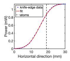
Figure D.8: Knife-edge measurements (blue circles) along vertical (left) and horizontal (right) directions at the intermediate plane of the imaging beam; fit with an error function (red solid line) giving the central position of the beam; and position (black dashed line) of the atomic cloud. The total power, central position and waist fit values are 1.167(7) mW, 38.03(7) mm, 10.8(2) mm for the horizontal direction and 1.153(7) mW, 15.10(8) mm, 10.9(2) mm for the vertical direction.
