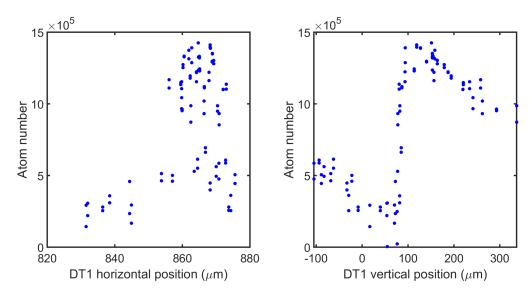
Figure B.26: Scan of the mirror verticality. The 0 on the x-axis is referenced to the in situ position of the magnetic trap. DT1 vertical position of  $-100\mu m$  means that DT1 is above MT by  $-100\mu m$ , and  $+100\mu m$  means that DT1 is  $100\mu m$  below MT.
