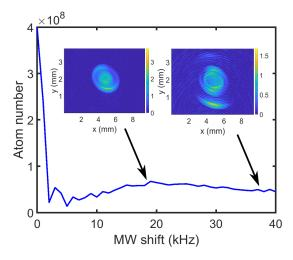
Figure B.14: Residual magnetic gradient inhomogeneties at the best compensation values.
