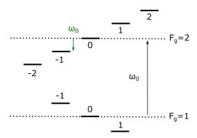
Figure B.7: Zeeman levels for the two hyperfine ground states shifted under a constant magnetic field.
