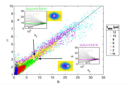
Figure D.12: Correction factor  $\alpha$  vs. the optical density for all MW datasets  $(2,4,6,8,10,12~\mu s)$ . Each point corresponds to 1 pixel and the solid line is a linear fit.
