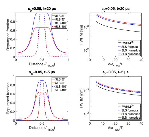
Figure E.7: Repumped fraction and FWHM for the repumper detuning tuned at the bottom of the modulation of  $F_e = 2$  as a function of the light shift of  $F_e = 2$ . The modulation interfringe is 8.3 µm. We show them for a pulse duration of 5 µs and 20 µs.
