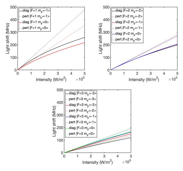
Figure E.4: Light shifts for a linearly polarized 1529.36098 nm laser for the states F = 1, F = 2 and F = 3 of  $5P_{3/2}$  vs. the 1529 intensity. Solid lines are the diagonalization ('diag') of the full Hamiltonian and dashed lines the perturbation theory ('pert'). All energies are referred to the hyperfine shift of the particular state considered.
