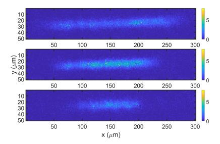
Figure A.3: Optical density from in situ absorption imaging for a DDS trap along the x-direction for top, middle and bottom of the excited state potential, s = 0.0005 and a trap depth of  $-14\Gamma$ . The DDS trap corresponds to the red curves of Fig. A.2.
