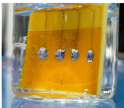
Figure II.16: Formation of an air layer around the structured ink electrodes in aqueous electrolyte, indicating a hydrophobic behaviour.
