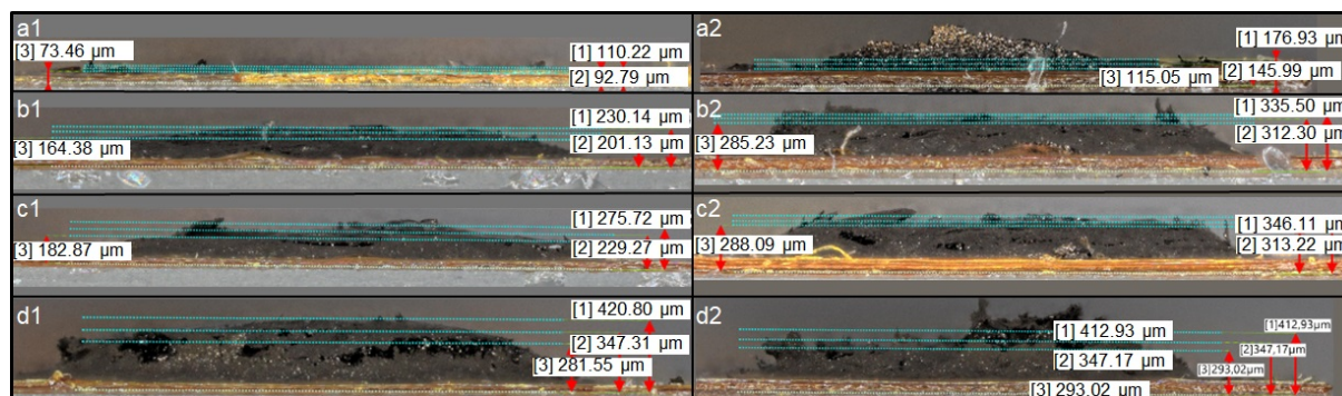
Figure III.44: Side view digital microscopy images of structured ink in the study of saturation temperature. 1 \mu\text{L} in series 1) and 1.5 \mu\text{L} in series 2). Sample 0/30 in a), 10/30 in b), 20/30 in c) and 30/30 in d).
