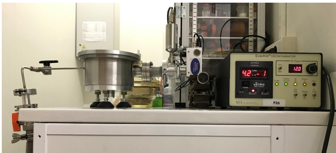
Figure 2. 7: The oxygen plasma instrument setup for cleaning the surface of the sample.
