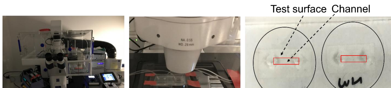
Figure 5. 5: Experimental setup for the dynamic observation of bacterial adhesion under flow, showing a testing surface with an integrated channel and the observation system on an optical microscope.
