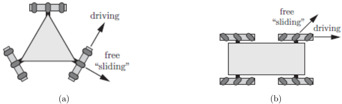
Figure 1.1: Holonomic Mobile Robots [Lynch and Park 2017]
