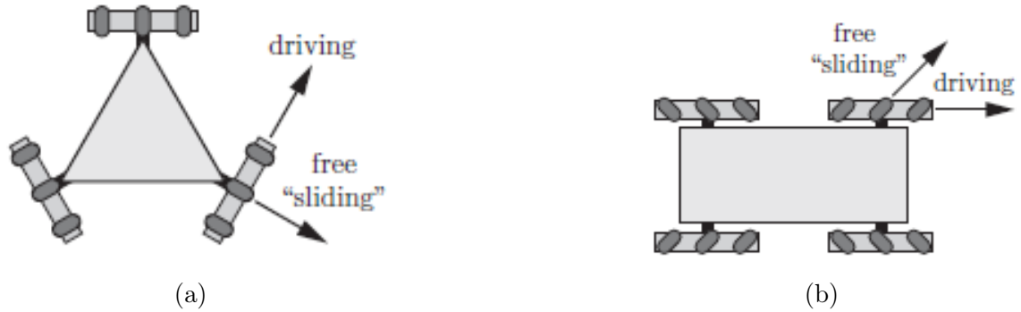
Figure 1.1: Holonomic Mobile Robots [Lynch and Park 2017]
