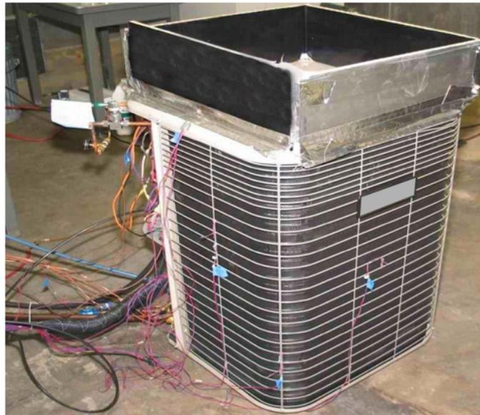
Figure 2.11: Side view of the outdoor section with the flow guide
