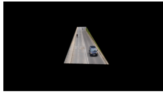
Figure C.4 – Detection Zone for extraction vehicle trajectories
