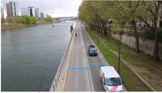
Figure C.3 – Detection lines for the count of different type of vehicles
