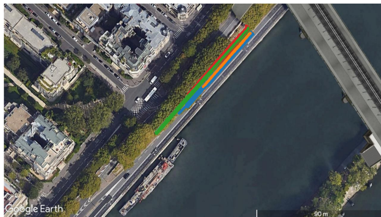
Figure C.8 – Vehicle trajectories extraction presented in the orthographic Google Earth image
