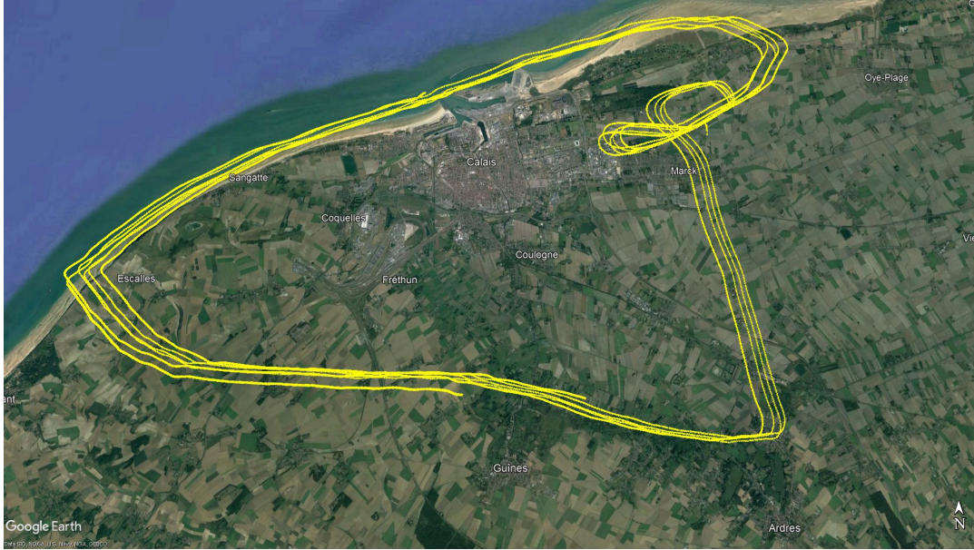
FIGURE 5.10: The satellite footprint traces along the flight trajectory imposed on Google Earth software. The traces of very low elevation satellites are not shown in the figure.
