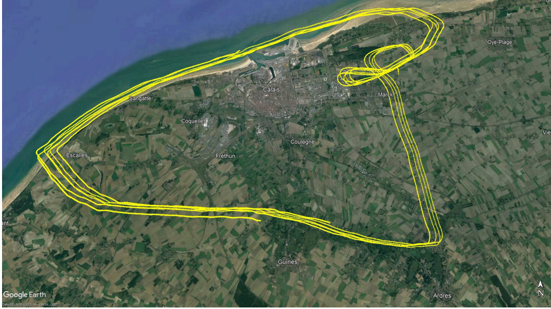
FIGURE 5.10: The satellite footprint traces along the flight trajectory imposed on Google Earth software. The traces of very low elevation satellites are not shown in the figure.
