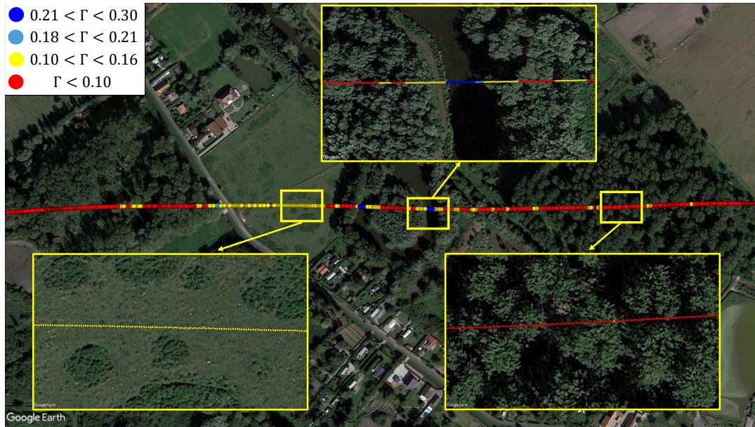
FIGURE 5.18: Surface differentiation using the GNSS measurements obtained from PRN 30 satellite signals.
