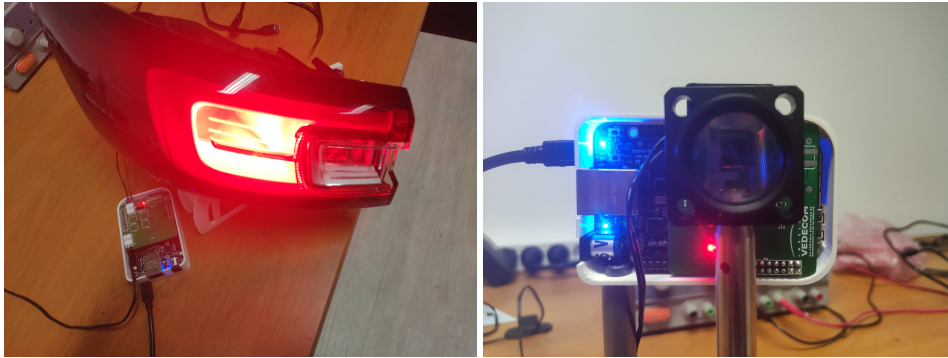
(a) Vehicular VLC Tx integration (b) Vehicular VLC Rx platform
