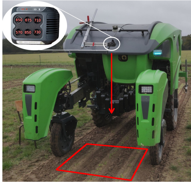
Figure 5.4 – The experimental set-up : the multispectral camera and the robotic platform
