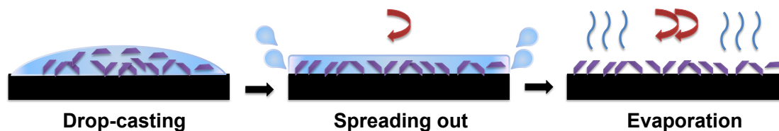
Figure 4.6: Schematic representation of the process of spin-coating.
