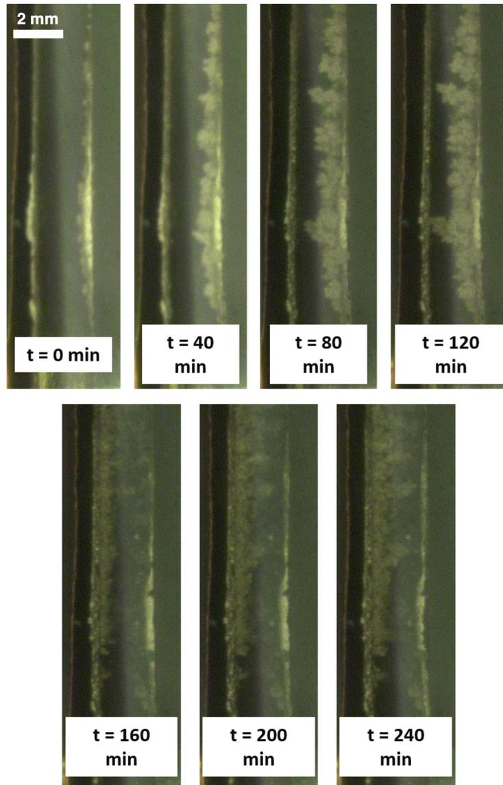
**Figure 5.27:** Images recorded by optical microscopy during a lithium stripping/plating experiment on a cell with the carbonates-based electrolyte.  $1 \text{ mA}\cdot\text{cm}^{-2}$  was applied to the cell for 2 hours, followed by  $-1 \text{ mA}\cdot\text{cm}^{-2}$  for the same amount of time.
