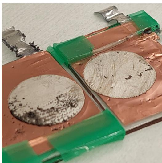
**Figure 5.29:** *Post-mortem* images from the same cell presented in Fig. 5.27. The electrode on the left corresponds to the electrode on the left in Fig. 5.27 (same correspondence for the electrode on the right).
