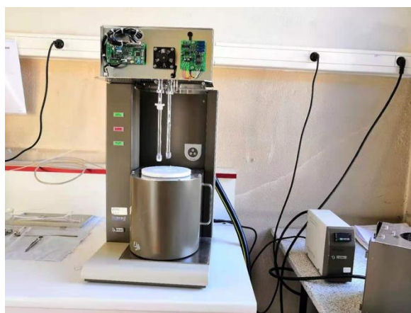
Figure. 3.6. BELSORB MINI Apparatus used in the physical adsorption of nitrogen (N 2 ).
