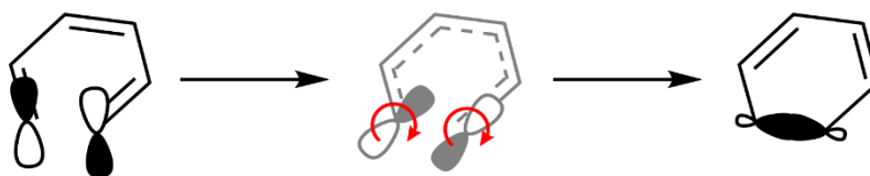
Figure 25: Light-induced conrotatory cyclization of 1,3,5-hexatriene to cyclohexadiene
