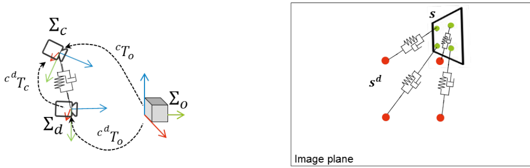
Figure 5.1 – Desired mass-spring-damper behavior in the case of 3D pose (left) and four image point visual features (right). The current \Sigma_c and desired \Sigma_d camera frames are sketched as well as the object frame \Sigma_o . The current \mathbf{s} (green) and the desired \mathbf{s}^d (red) image point features in the image plane are depicted. The target is arranged in a coplanar square shape.
