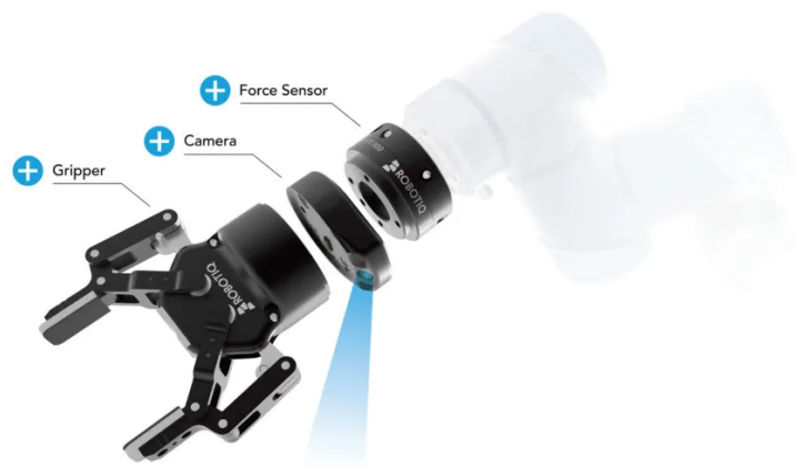
Figure 4.6 – Robotiq integrated solution for cascading wrist-mounted Force/Torque sensor, vision system and two finger gripper designed for the Universal Robots.
