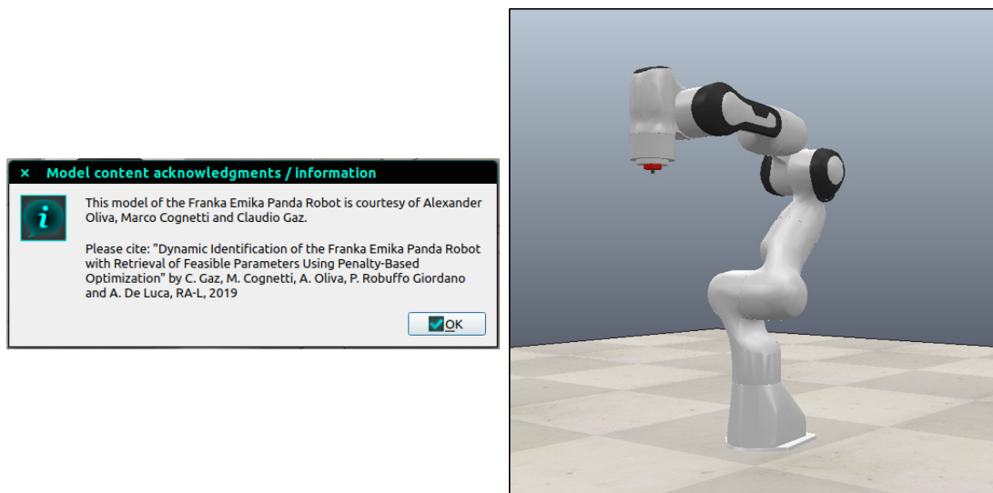
Figure 7.5 – The Franka Emika Panda robot in Coppeliasim. The released model is available by default since the version V4.0.0.
