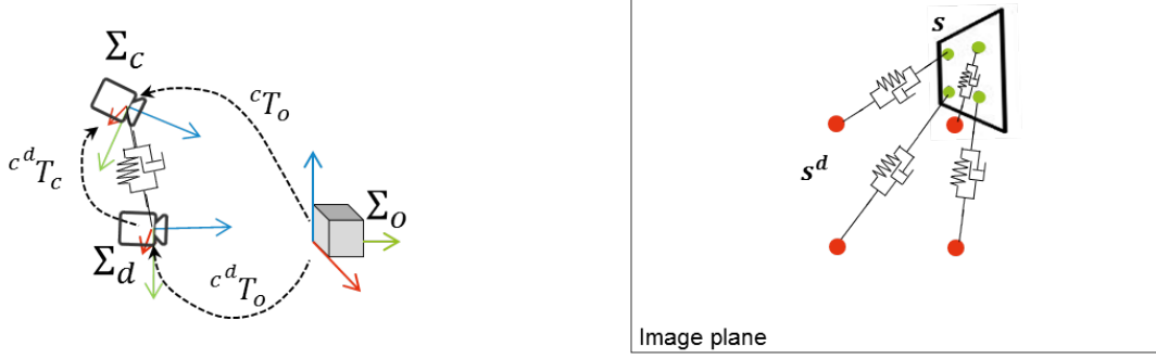
Figure 5.1 – Desired mass-spring-damper behavior in the case of 3D pose (left) and four image point visual features (right). The current \Sigma_c and desired \Sigma_d camera frames are sketched as well as the object frame \Sigma_o . The current s (green) and the desired s^d (red) image point features in the image plane are depicted. The target is arranged in a coplanar square shape.
