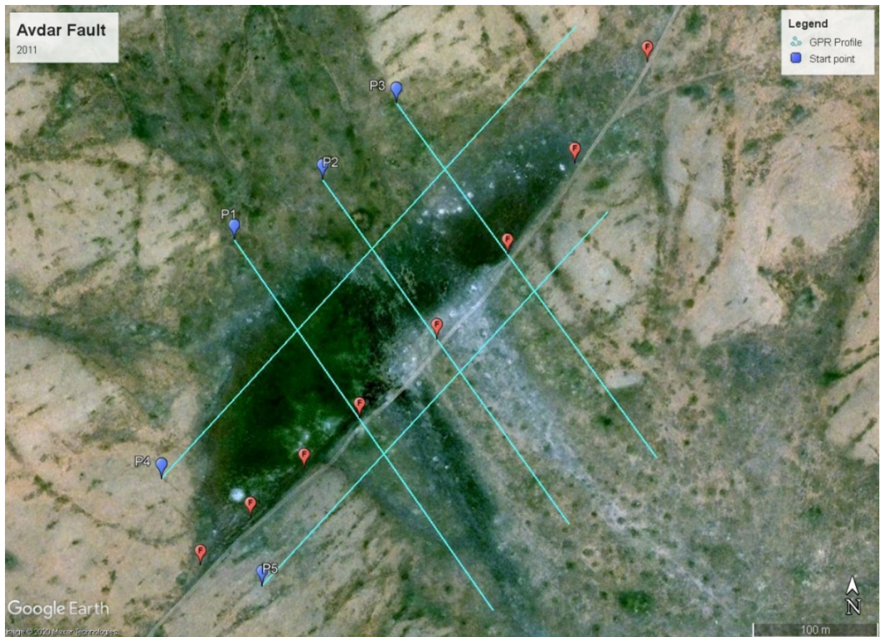
Figure 2.24 Location map of ground penetrating radar profiles in Z2 zone. The zone location is shown in Figure 2.23. Light blue lines indicate the profiles at the RTA50 MHz, 500 MHz and 250 MHz antenna. The blue symbols are indicating the start points and name of profiles. The red symbols are representing fault trace.
