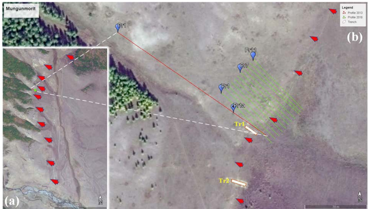
Figure 2.12 Location map of GPR profiles on the Mungunmorit active fault. a) Main location of GPR and trench study, red arrow is fault trace. b) GPR profiles and trench location, red line is GPR profile in 2013, green line is GPR profile in 2016, white square is paleo seismological trench, blue symbol is profile name and start point.
