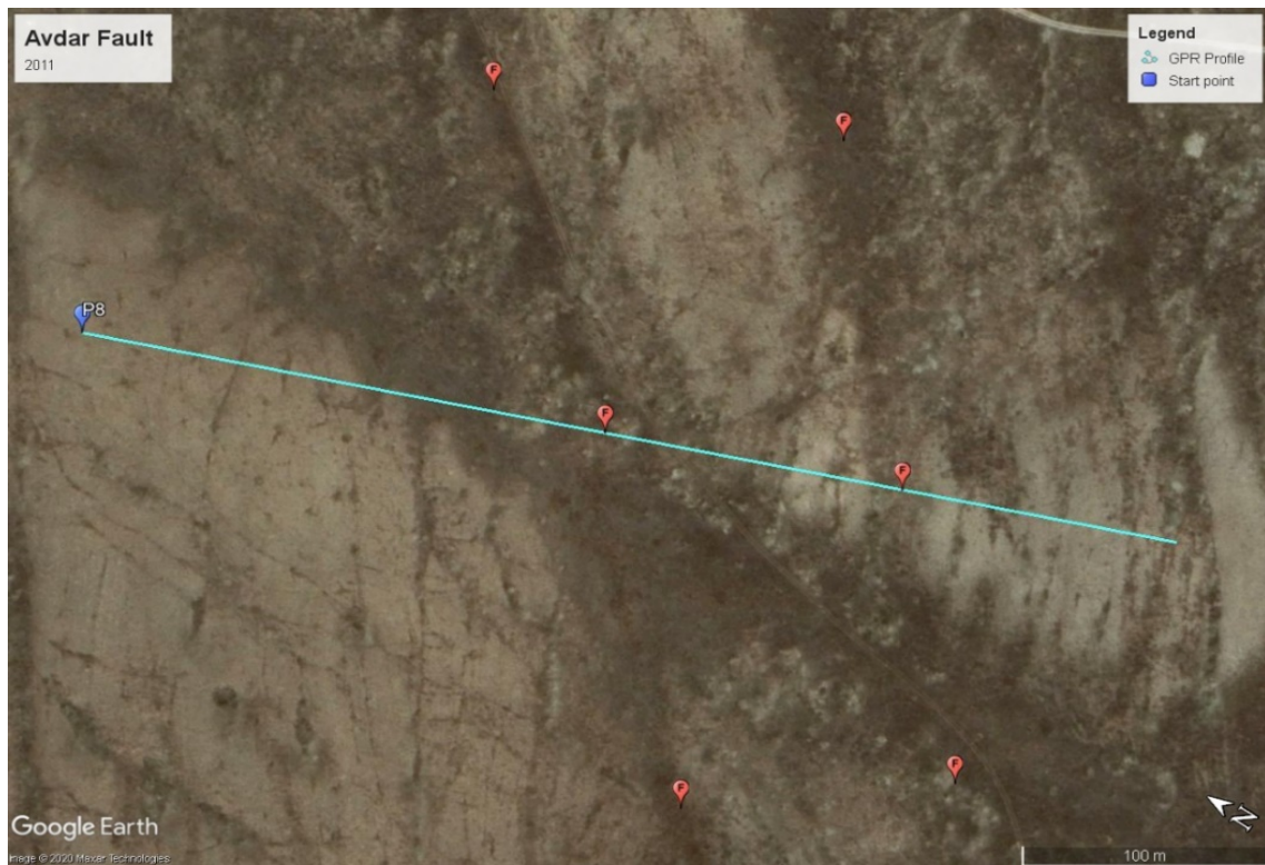
Figure 2.26 Location map of ground penetrating radar profiles in Z1 zone. The zone location is in Figure 2.23. Light blue lines indicate the profiles at the RTA50 MHz, 500 MHz, and 250 MHz antenna. The blue symbols are indicating the start points and name of profiles. The red symbols are representing fault trace.
