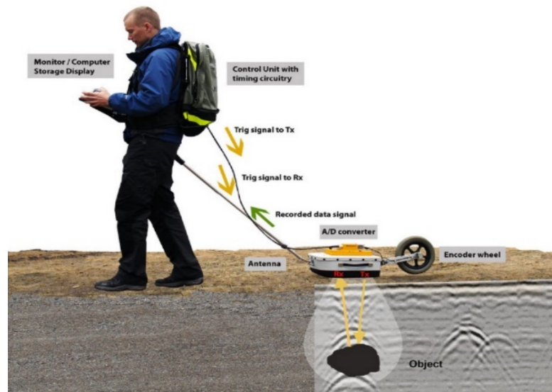
Figure 1.5 The different components of a GPR system. Image Source: (Canada: Geoscan)
