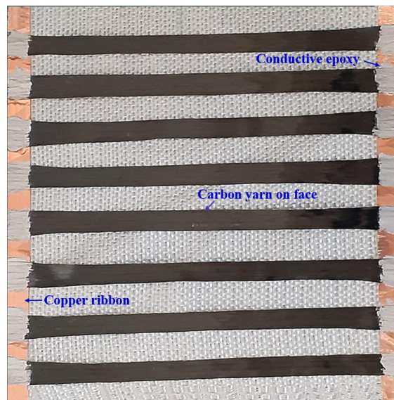
Figure 27: Illustration of carbon yarn insertion on one side SNC
