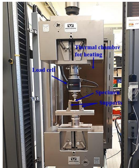
Figure 43: Experimental set up of three-point bending tests of SMP composite specimens in a thermal regulating chamber
