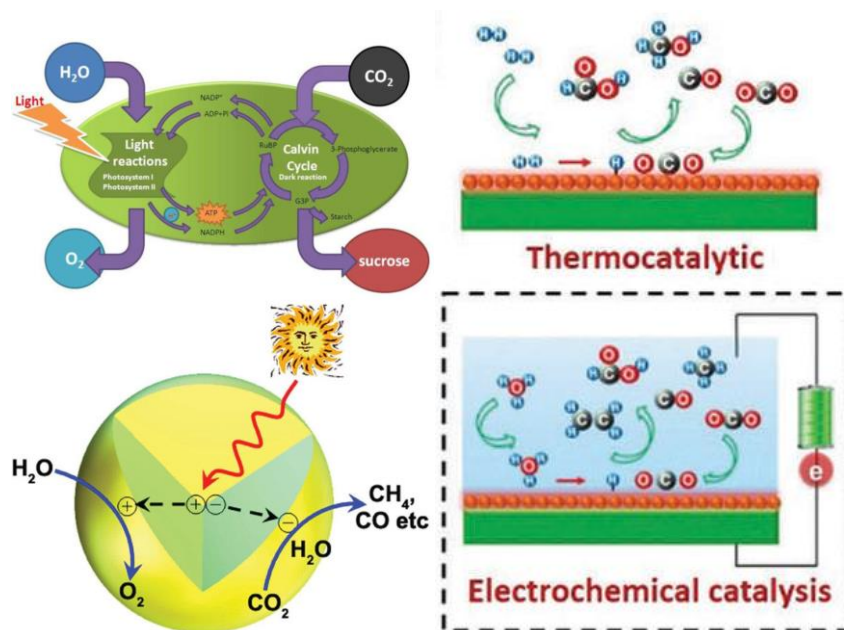
Figure 1.1. Typical processes of CO 2 conversion: photosynthesis, photocatalysis, thermocatalytic and electrochemical catalysis. Reproduced with permission [16]. Copyright 2017, the RSC.
