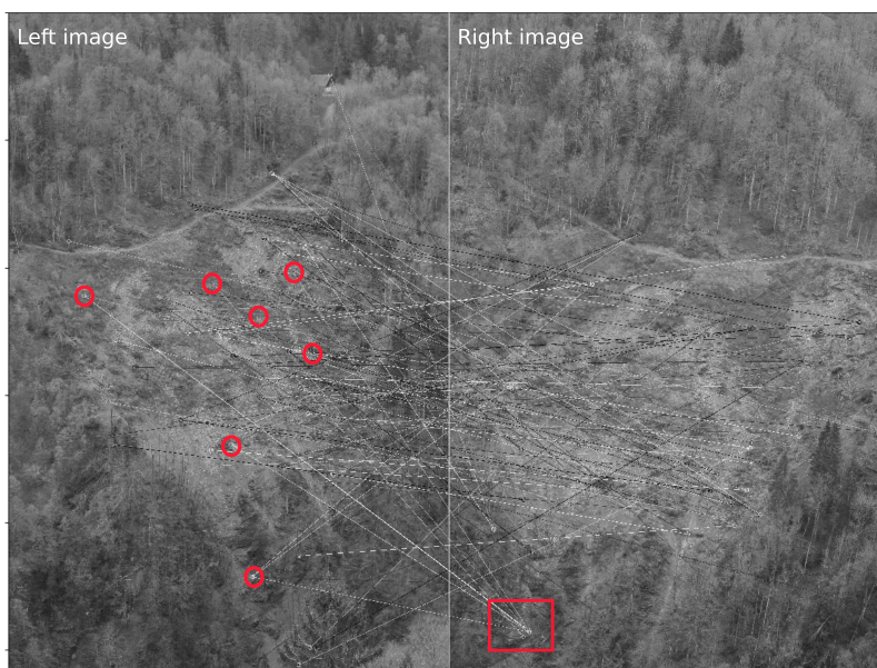
Figure 3.5: Image pairing by using the ORB detector. 171 features are detected for the pair-image acquired the February 11 2020. Drawn lines connect the pairs of homologous points. As we can noticed with the red circles and the red rectangular, several features from one image get the same homologous point in the second image and conversely.
