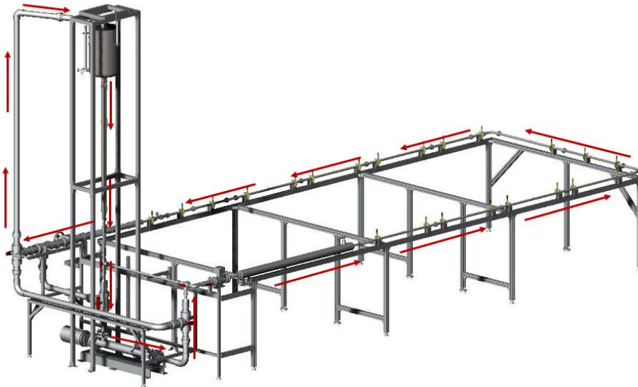
Fig. 2.5 Fluid circuit in the hydraulic loop.
