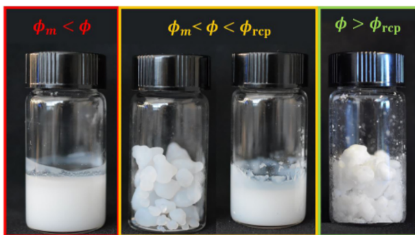
FIG. 3. Result of mixing suspensions of silica particles at different mass fractions \phi^{\text{wt}} . From left to right, the first vial corresponds to \phi^{\text{wt}} < \phi_m^{\text{wt}} with and without vibrations (here, \phi^{\text{wt}} = 23 \text{ wt. \%} and vibrations are not applied). The second and third vials correspond to \phi_m^{\text{wt}} < \phi^{\text{wt}} < \phi_{\text{rcp}}^{\text{wt}} (here, \phi^{\text{wt}} = 29 \text{ wt. \%} ), without vibrations (second vial) or when vibrations are continuously applied during mixing (third vial). The last vial corresponds to \phi^{\text{wt}} > \phi_{\text{rcp}}^{\text{wt}} with and without vibrations (here, \phi^{\text{wt}} = 30 \text{ wt. \%} and vibrations are applied). The studied suspension is characterized by \phi_m^{\text{wt}} \simeq 0.24 and \phi_{\text{rcp}}^{\text{wt}} \simeq 0.3 .
