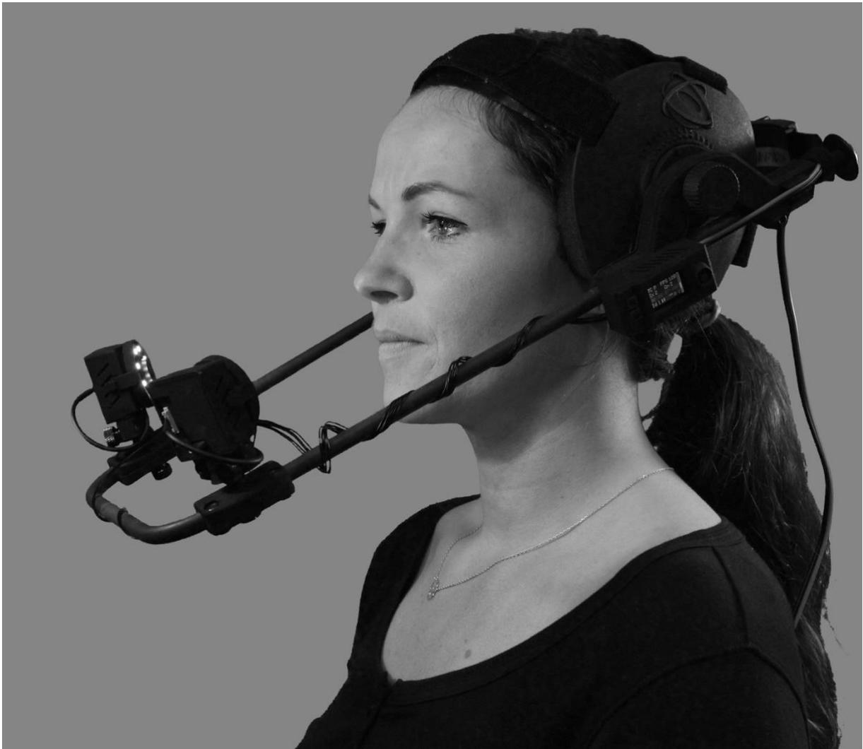
**Figure 3:** facial motion capture with Dynamixyz.
