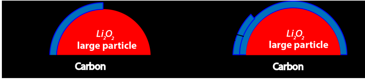
Figure 3.2: Schematics of the \text{LiO}_{2(s)} formed on the surface of a large \text{Li}_2\text{O}_2 particle: To the left, a case is represented where the \text{LiO}_{2(s)} monolayer covers less than the large \text{Li}_2\text{O}_2 particle surface ( \theta < 1 ), and to the right, a case is represented where \text{LiO}_{2(s)} completely covers the large \text{Li}_2\text{O}_2 particle surface and forms a multilayer ( \theta = 1 ).
