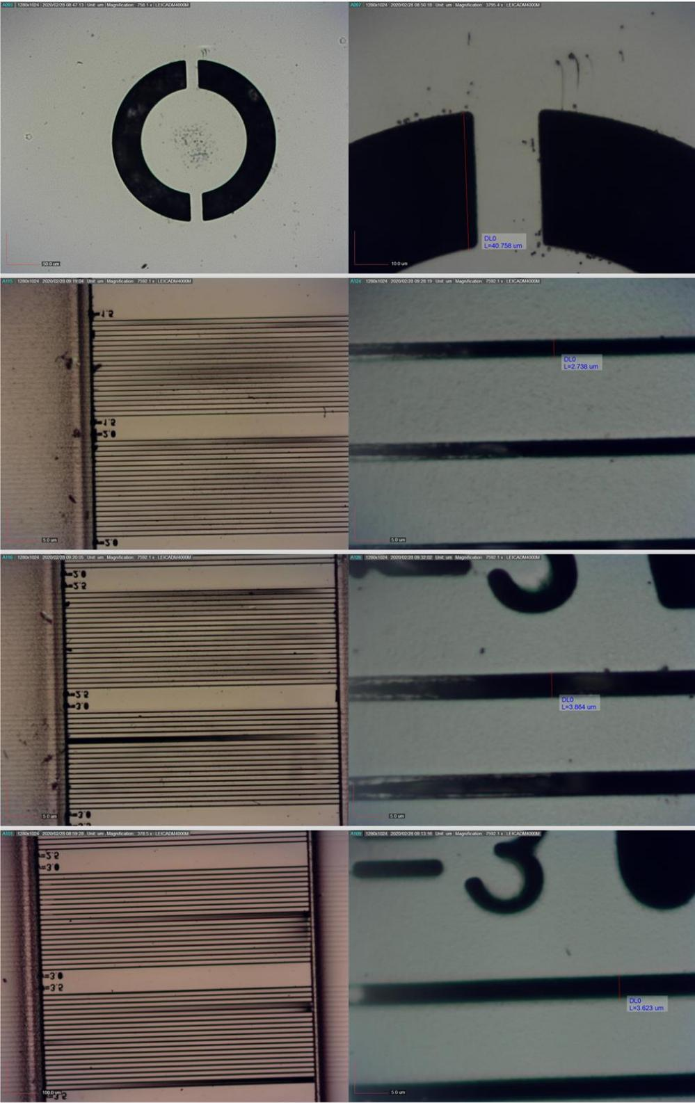
**A4.3 Representative SEM graphs of patterned 100 nm thick Al deposited on glass substrate.**
