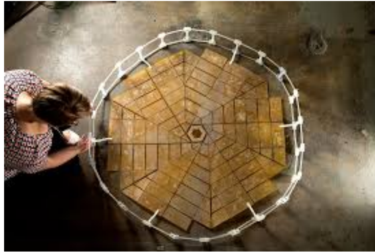
FIGURE 1.4: A 1/20th-scale tabletop prototype (expands to a deployed diameter of 1.25 meters) of the Origami-based solar panel array developed by NASA using the origami Patten called the “ flasher ” [Landau, 2014].
