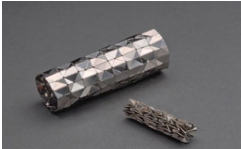
FIGURE 1.9: An origami-based stent-graft in its folded and deployed states [Kuribayashi et al., 2006].
